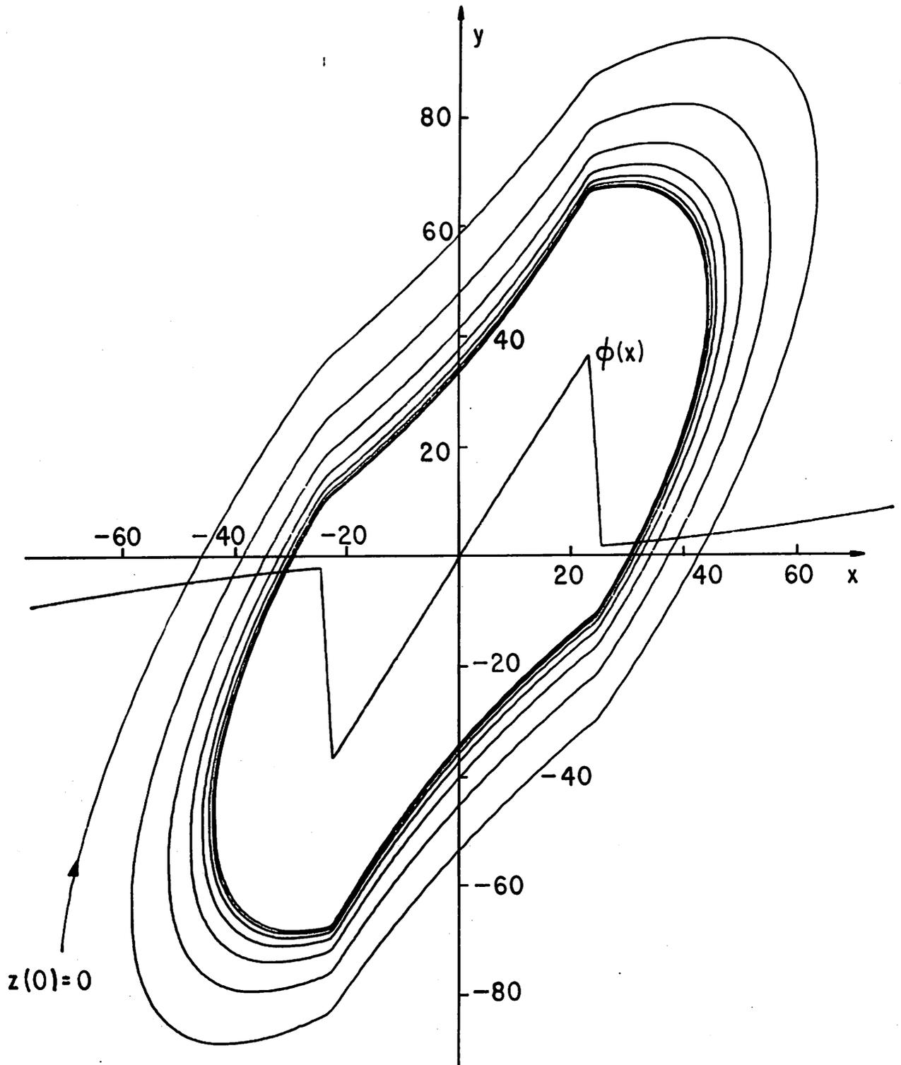
Fig. 2. Projection on the plane  $z = 0$  of a trajectory approaching the stable limit cycle.
