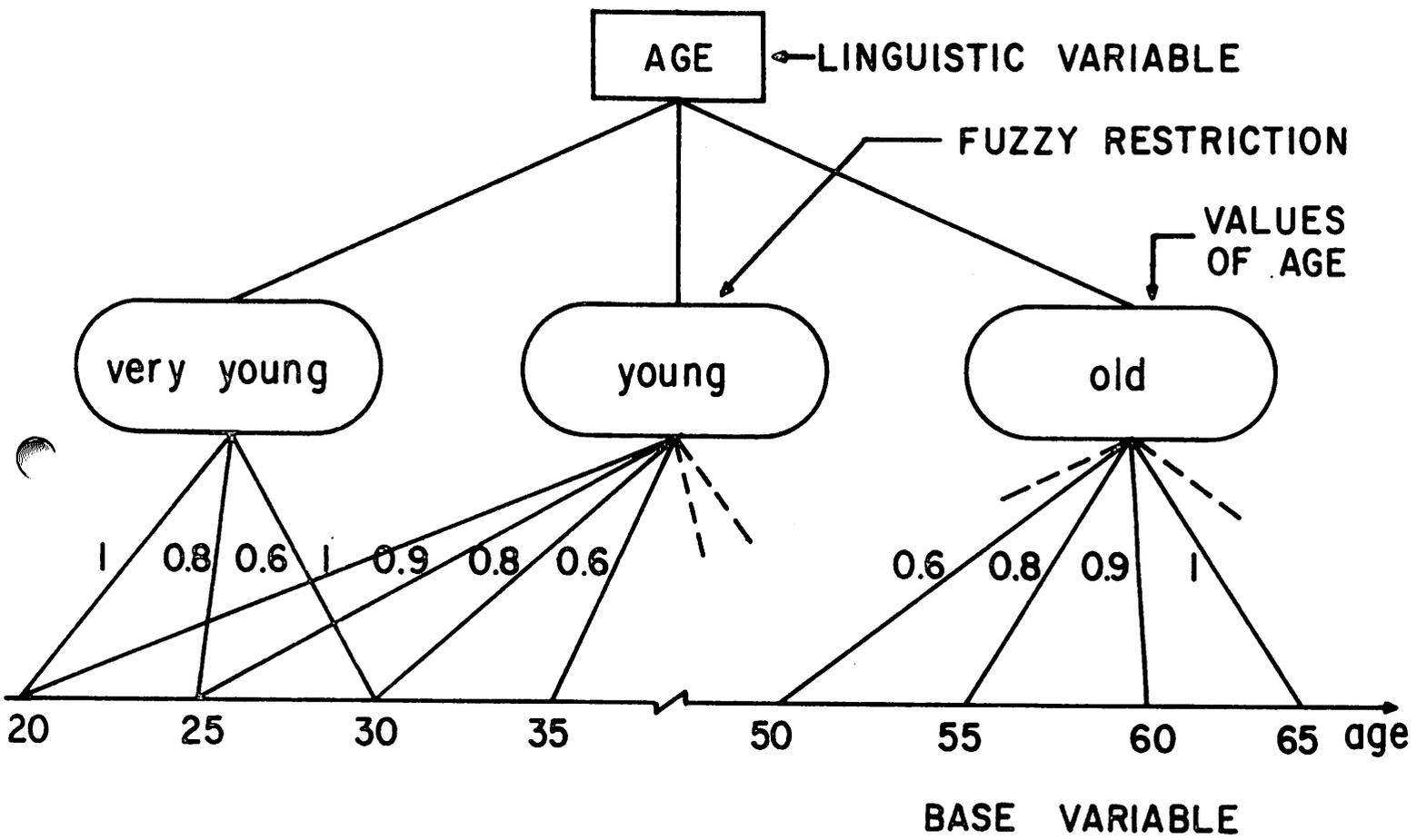
Fig.1.3. Hierarchical structure of a linguistic variable.
