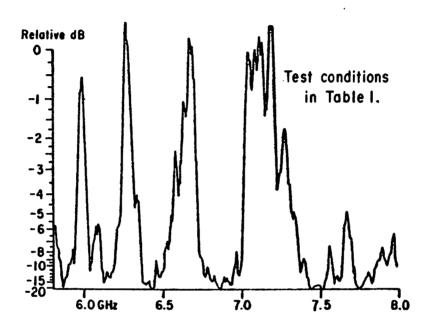
Fig. 6. Swept-frequency backscatter taken at 39° incidence, at 14:15, 3/3/77.
