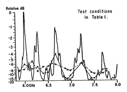
Fig. 7. Dependence of backscatter on amount of signal frequency modulation.
