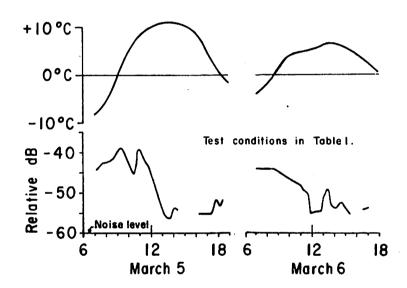
Fig. 1. Fixed-frequency backscatter as a function of temperature and time of day.
