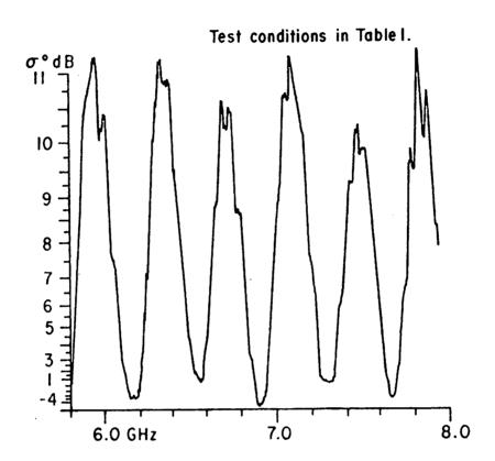
Fig. 4. Swept-frequency backscatter taken at 0° incidence at 13:07, 3/5/77.
