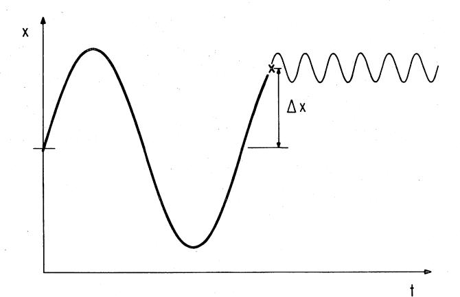
FIGURE 2. An illustration of the transport process responsible for the dissipative trapped electron instability. At  $\searrow$  the trapped electron suffers a collision and scatters into a passing orbit. This results in a "step",  $\Delta x$ , and a momentum transfer between the electron distribution and the wave in the amount  $\Delta p_y = eB\Delta x$ .
