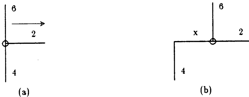
Figure 15: Numbers indicate segment widths. (a): Initial Position. (b): Final Position. The width of the segment labeled x should be 4.
