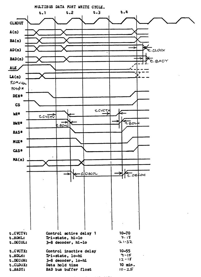
Meets data set up and hold times for AMD 2953.
