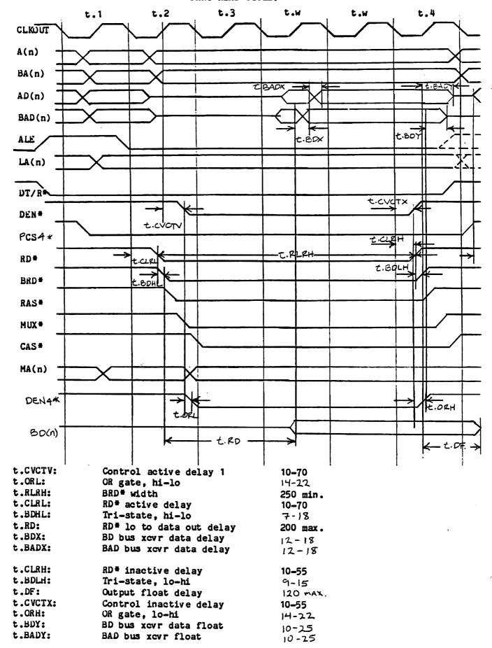
Meets data set up and hold times for '186. Meets '186 data float before next address.
