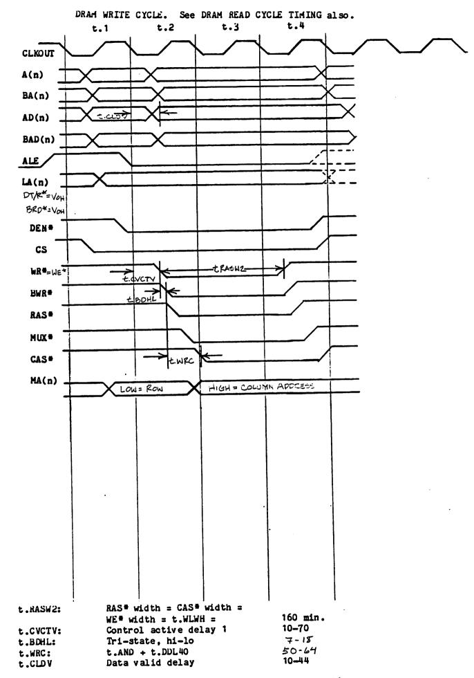
Meets DRAM data set up time. Meets write command set up time.
