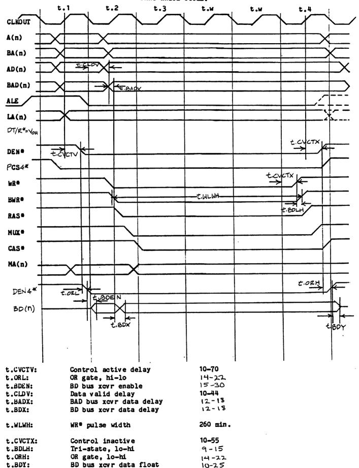
Meets data set up and hold times for 8274 DART chip.
