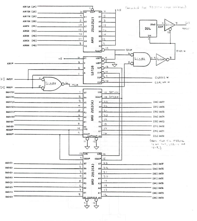
MULTIBUS ADDRESS DECODE
