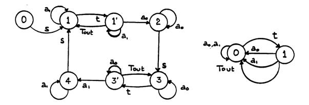
Thus transmissions  $t_0$  and  $t_1$  are enabled only in states 1 and 4 respectively, so that a timeout (Tout) or a valid acknowledgement must occur between successive transmissions.
