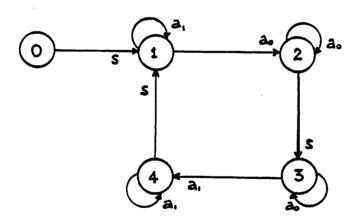
Supervisor  $S_2$  observes G through  $M_2$  and controls  $\Sigma_{2,c}$ . It has the four state automaton  $S_2$  shown in the sketch below and the feedback rule
