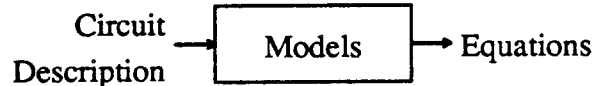
Figure 2. A performance model is a template for producing equations that specify design performance metrics, given a circuit description (e.g. a net-list).
