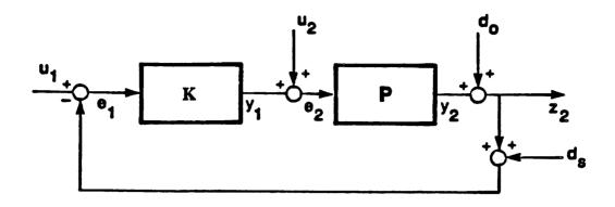
Figure 1: The feedback system S(P,K).
