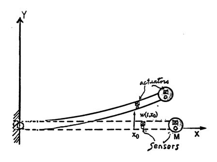
Figure 2: Planar bending motion of a flexible beam.
