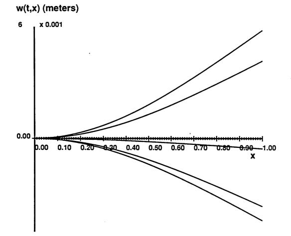
Figure 6. Variation of Beam Profile with Time
