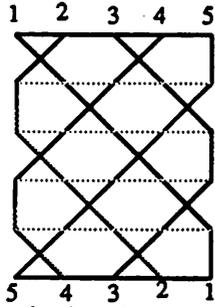
Figure 5. Routing by odd-even transposition
