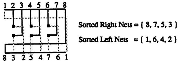
Figure 13. Routing in the overlap model
