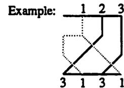
Figure 10b. 3-terminal subnet with two destination points are transformed into two 2-terminal subnets by introducing a pseudo terminal
