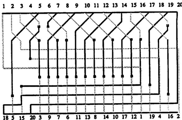
Figure 17. A channel is routed by the hybrid router in density.
