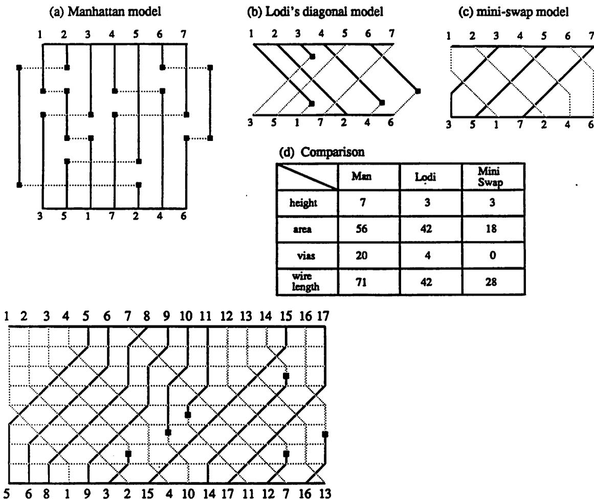
Figure 9. A channel with density = 7 is optimally routed in the mini swap model.
