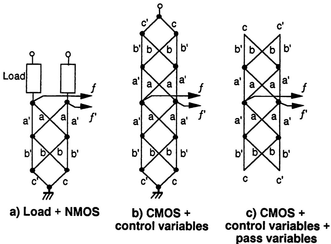
Fig.2 An example of MOSTL (a parity generator circuit)
