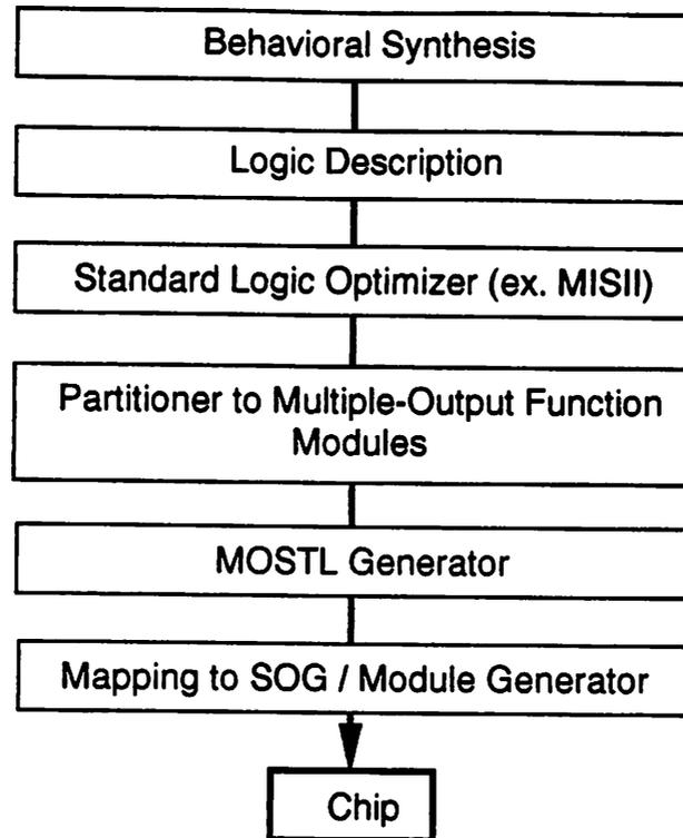
Fig.9 MOSTL generator incorporated in a design system
