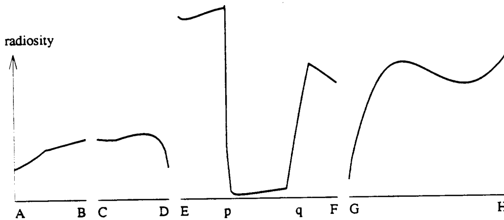
Figure 3.2: Radiosity as a function of arc length along the non-black edges of test scene. Note the sharp shadow edge at p and the gradual one at q.
