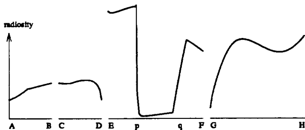
Figure 2: Radiosity as a function of arc length along the non-black edges of test scene. Note the sharp shadow edge at p and the gradual one at q .
