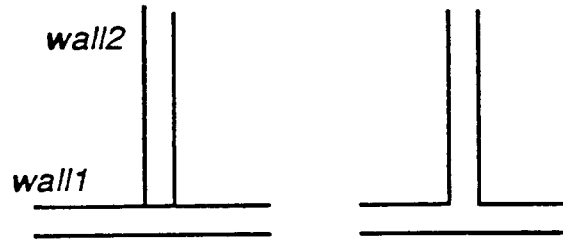
(a)Incorrect and (b)correct intersection Figure 4.2
