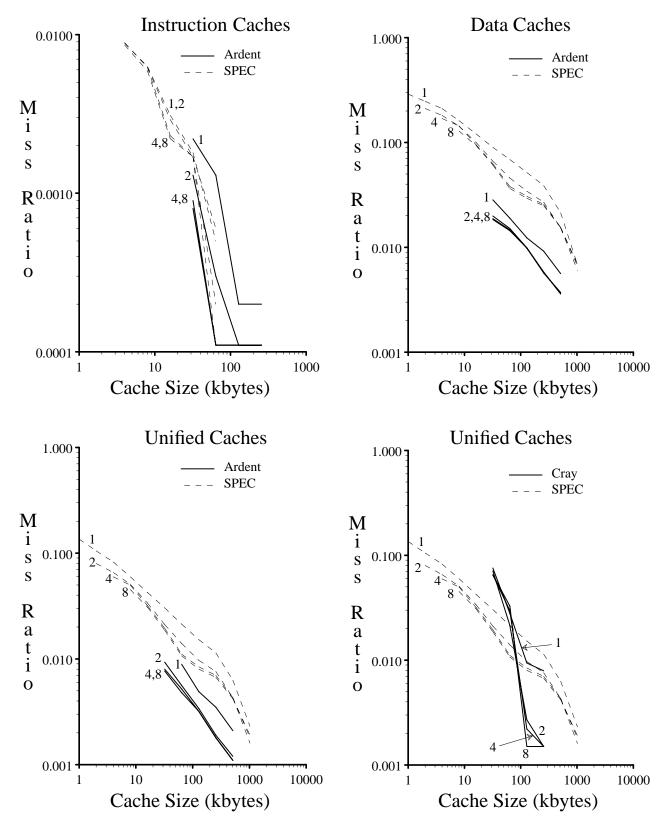
**Figure 6**: Set-associative Ardent and Cray cache miss ratios for a 64 byte block size, plotted against SPEC floating point miss ratios. Curves are labeled by set size.
