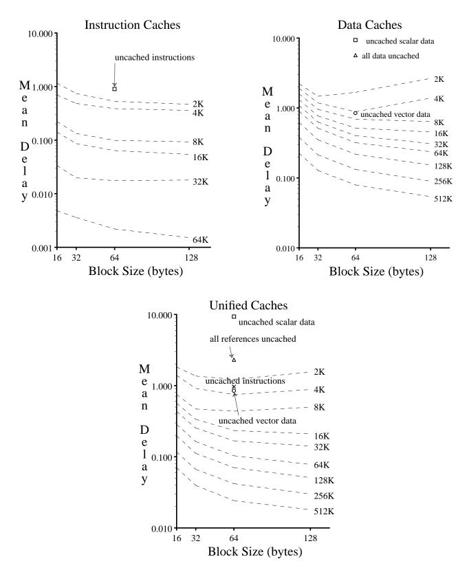
**Figure 8**: Mean delay per memory reference (cycles) for Ardent fully-associative instruction, data, and unified caches. Plots are labeled by cache size (Kbytes), and delays without caches are also shown for the different reference types. Memory latency is 14 cycles, and transfer time is 1 cycle per 8-byte word.
