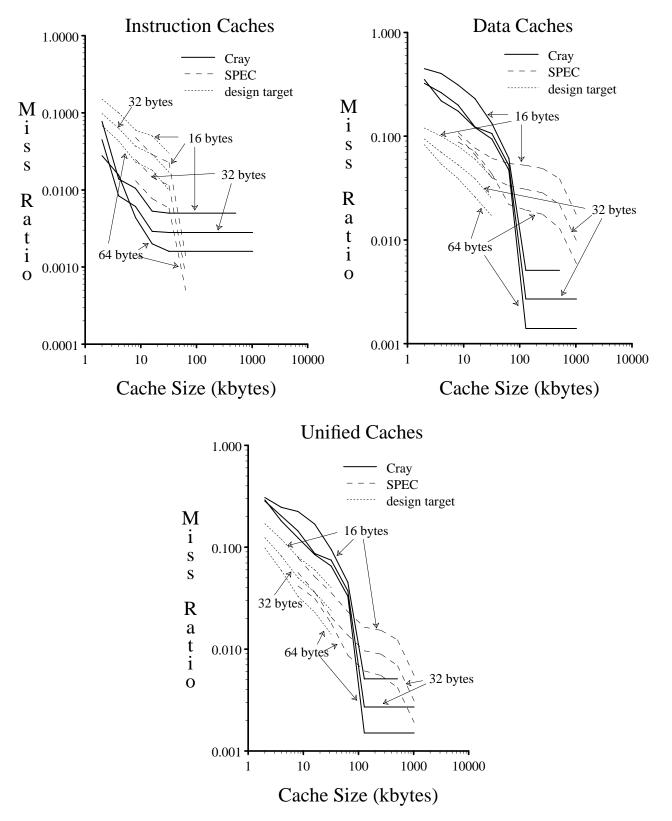
**Figure A7**: Fully-associative Cray vs. design target and SPEC floating point miss ratios. Curves are parameterized by block size.
