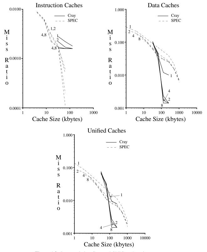
Figure A8: Set-associative Cray and SPEC cache miss ratios for a 64 byte block size. Curves are labeled by set size.
