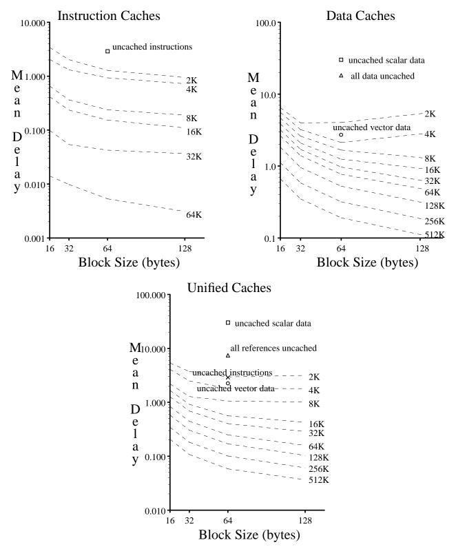
**Figure 9**: Mean delay per memory reference (cycles) for Ardent fully-associative instruction, data, and unified caches. Plots are labeled by cache size (Kbytes), and delays without caches are also shown for the different reference types. Memory latency is 45 cycles, and transfer time is 1 cycle per 8-byte word.
