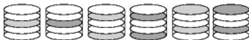
P+Q Redundancy (RAID Level 6)
