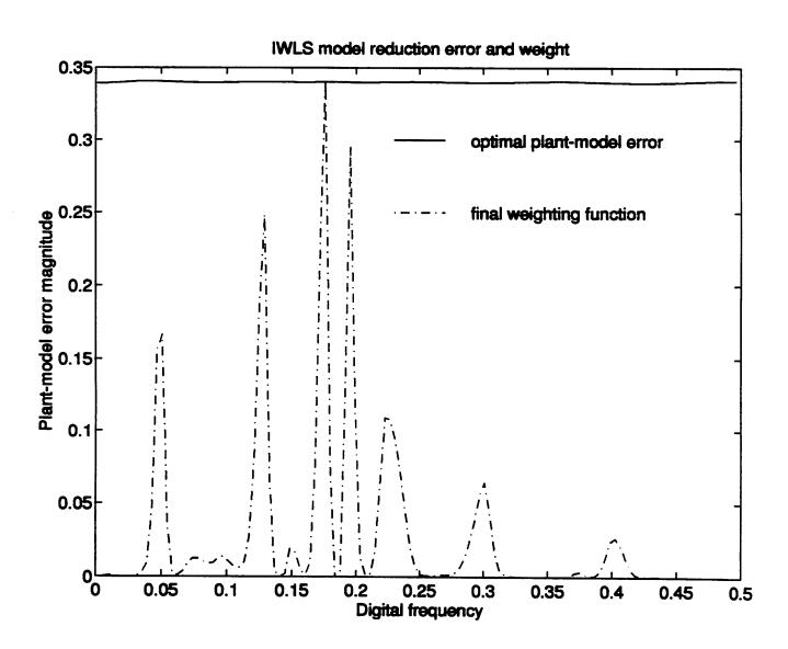
Figure 2: Minimum error and optimal weight magnitude
