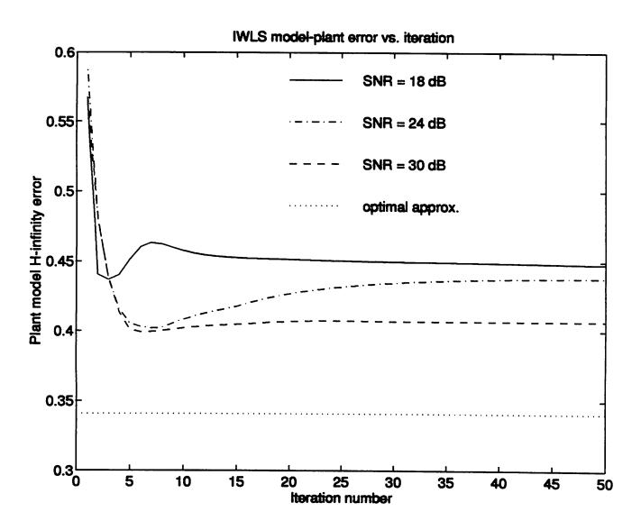
Figure 3:  $\mathbf{H}^{\infty}$  plant model error vs. iteration in IWLS algorithm
