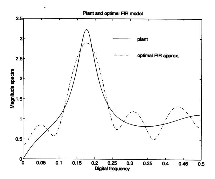
Figure 1: Plant and optimal FIR model approximation magnitude spectra
