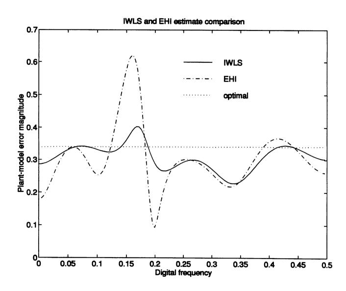
Figure 4: Typical plant-model error magnitude for IWLS and MR estimates. SNR = 22 dB.
