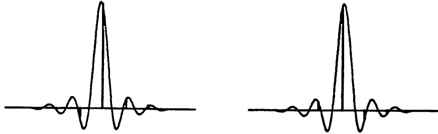
Figure 15. Positive and negative timing phase error for received isolated pulse with a zero-forcing equalizer. The equally spaced samples also represent the equivalent discrete-time channel and ISI. For \tau > 0 pre-cursor ISI is negative and the post-cursor contribution is positive. The situation is reversed in the case of \tau < 0 .
