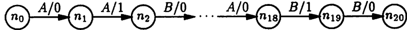
Figure 2.3: A specification for the behavior in Figure 2.1: each node will be part of some state in the minimal machine. Each transition is labeled with its input/output.
