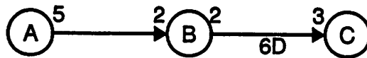
Figure 3. An SDF graph used to illustrate GDPPO applied to SDF graphs that have nonzero delay on one or more edges. Here q(A, B, C) = (6, 15, 10) .
