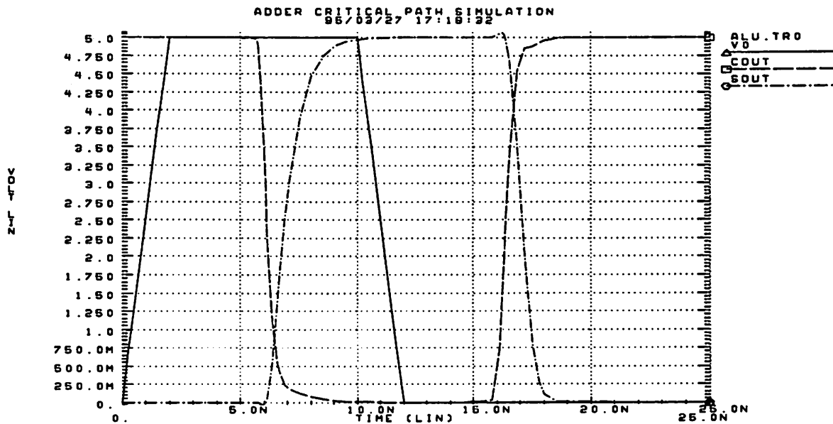
Figure 5-6: SPICE Critical Path Simulation of 16-bit Carry-Select Adder.
