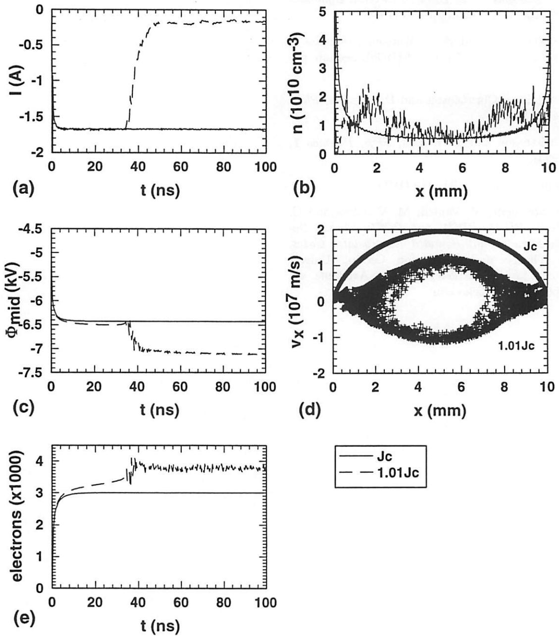
Figure 1: Crossed-field diode for Case A, the critical point (solid curves), and for Case B, at 1% above the critical point in injected current (dashed curves).
