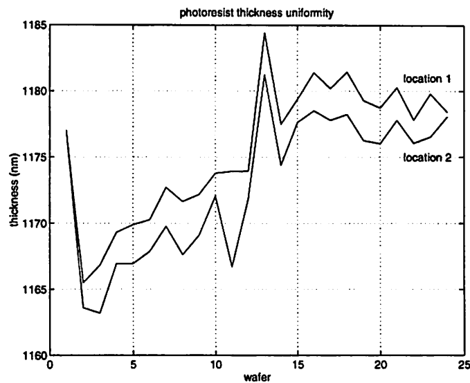
FIGURE 5 Photoresist thickness variation within wafer.
