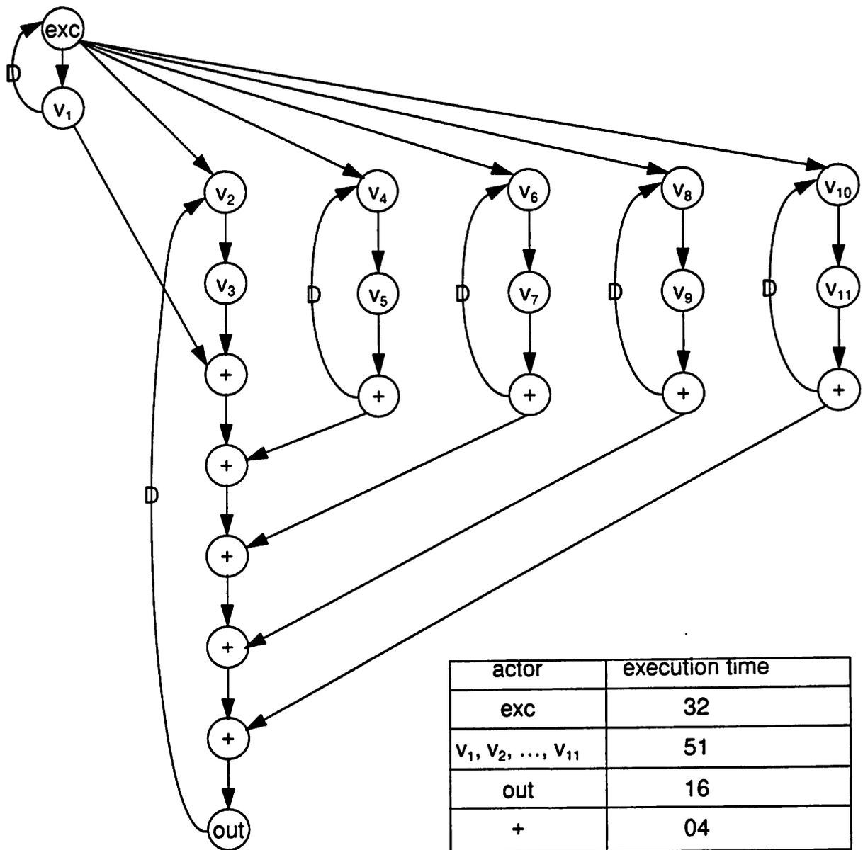
Figure 22. The synchronization graph that results from a six processor schedule of a music synthesizer based on the Karplus-Strong technique.
