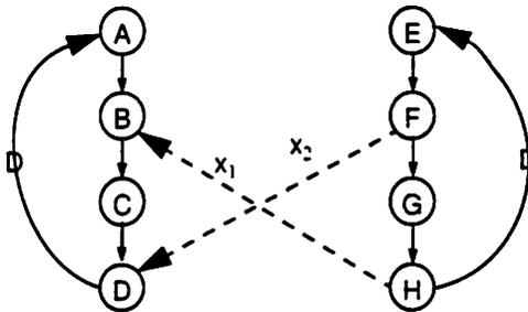
Figure 2. An example of a redundant synchronization edge: the edge  $x_2$  is redundant.
