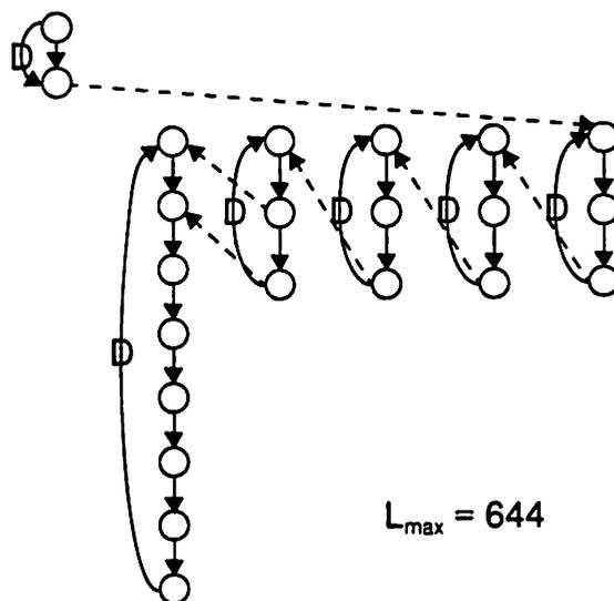
Figure 25. The synchronization graph computed by the heuristic for  $L_{max} = 644$ .
