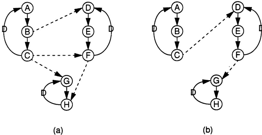
Figure 9. An illustration of a simple algorithm for optimal resynchronization of chainable synchronization graphs. The dashed edges correspond to synchronization edges.
