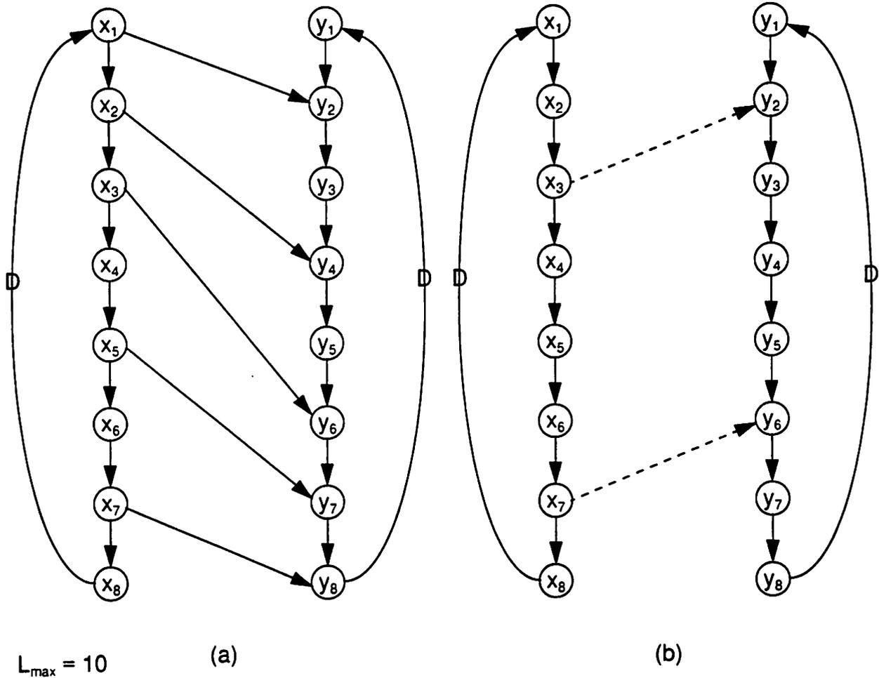
Figure 15. An instance of delayless, two-processor latency-constrained resynchronization. In this example, the execution times of all actors are identically equal to unity.
