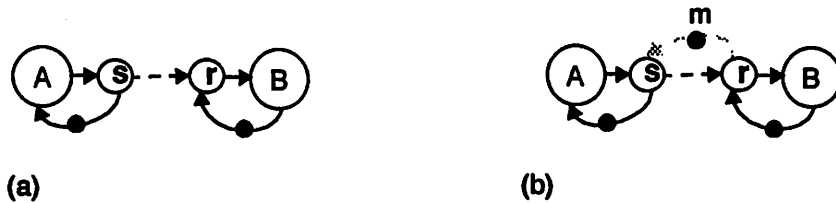
Figure 5.3. An IPC graph with a feedforward edge: (a) original graph (b) imposing bounded buffers.
