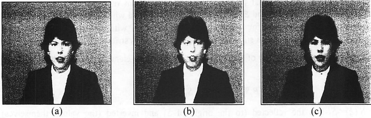
Figure 5. Example for the effect of the gray-scale erosion and dilation on gray-scale images. (a) is the original frame, (b) is the erosion, (c) is the dilation image. In the erosion image the brighter regions are emphasized and widened, while in the dilation image the darker regions are emphasized and widened.
