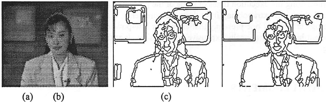
Figure 13. Comparison of compensated and uncompensated segmentation algorithms: input image (a), uncompensated output (b), and compensated output (c)
