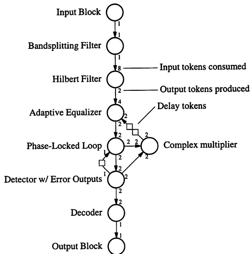
**Figure 2.13** An SDF description of a modem, adapted from Lee [41].
