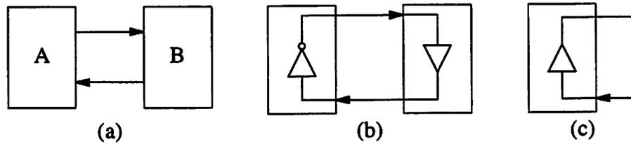
**Figure 1.2** Problems with zero-delay and feedback. (a) Co-dependent: Which should be evaluated first? (b) Paradoxical: Appears to have no solution. (c) Ambiguous: Appears to have many solutions.
