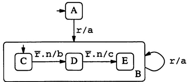
**Figure 2.7** The sequencer example described in Argos
