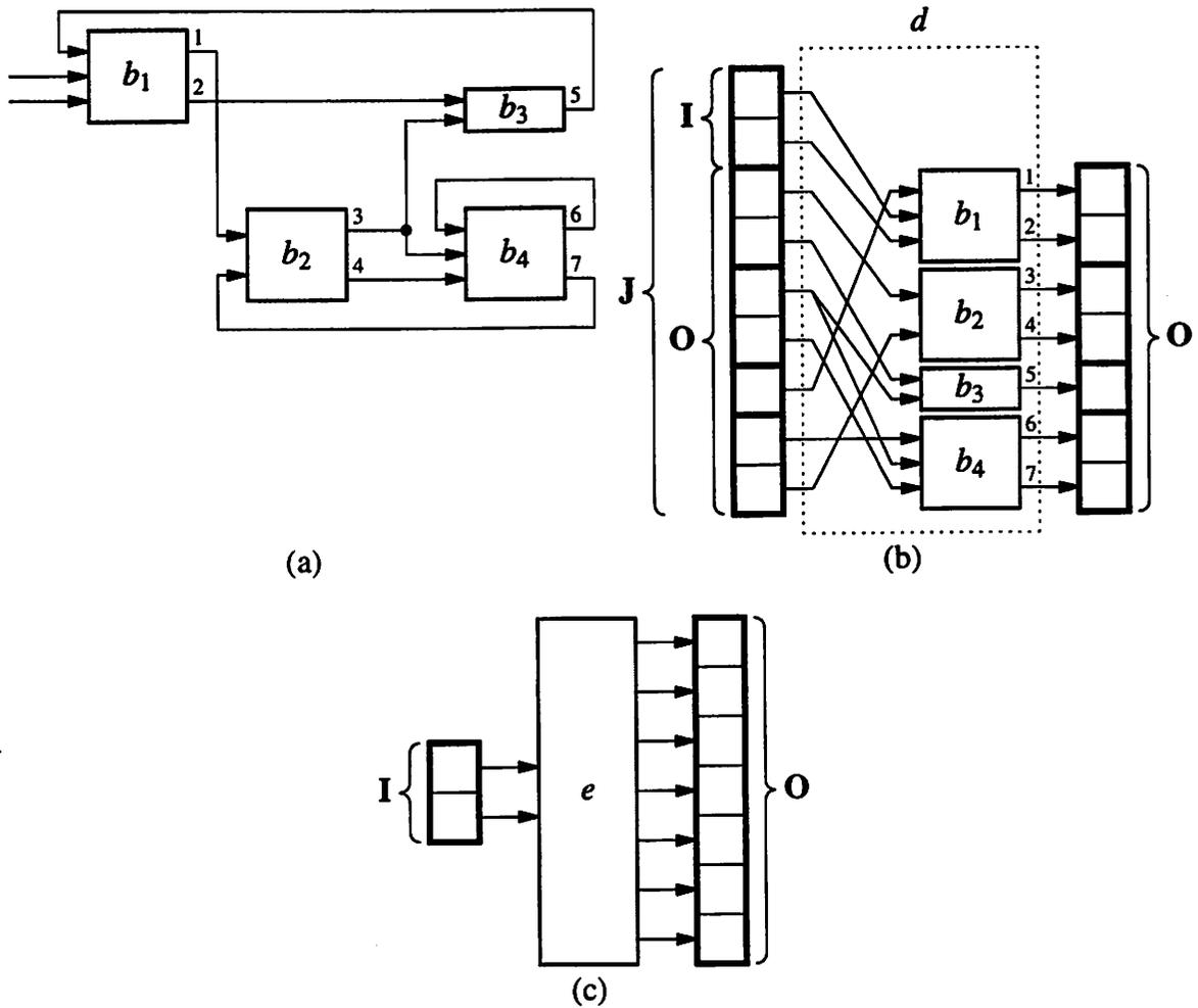
**Figure 3.6** (a) An SR system. (b) The corresponding open system. (c) The corresponding block.
