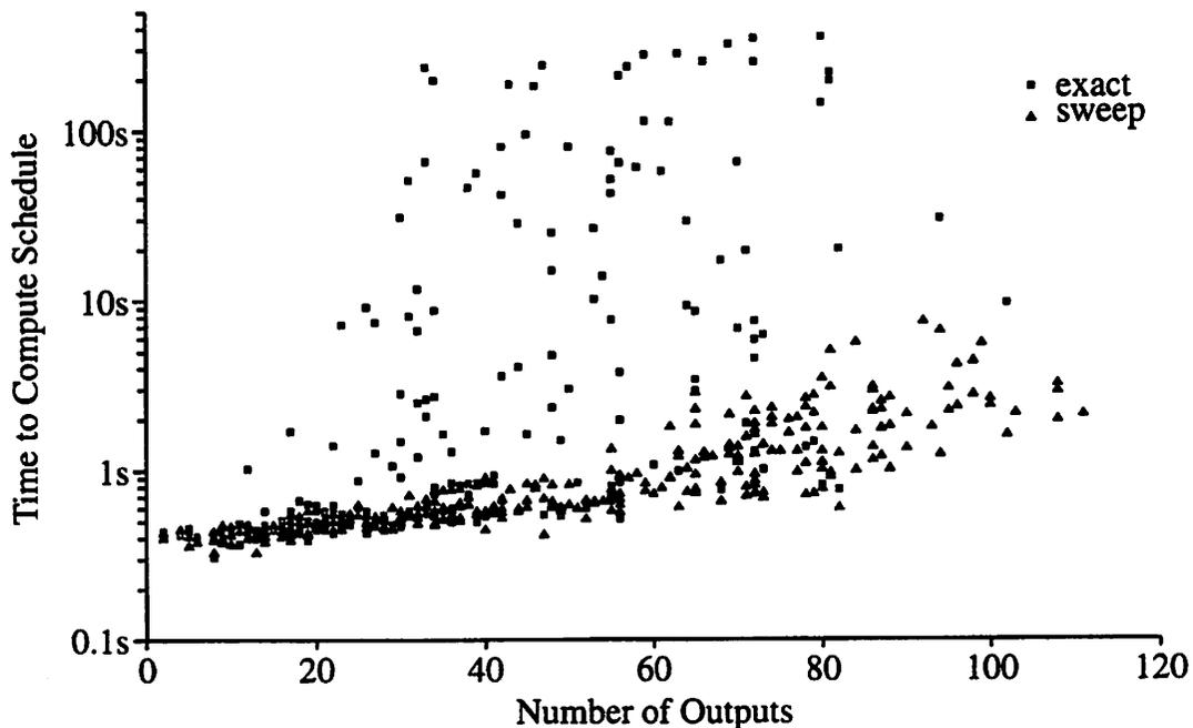
**Figure 4.18** A comparison of scheduling times for the branch-and-bound algorithm using the exact and heuristic sweep partition generators. All times are on a SPARCStation 10.
