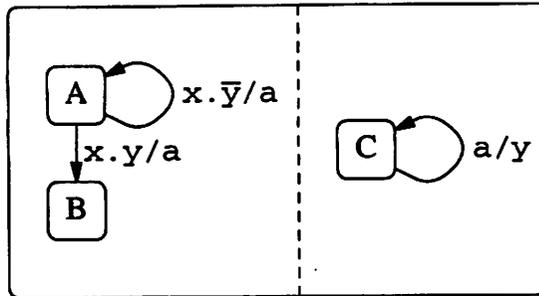
**Figure 2.8** Incremental behavior in an Argos program. When in State A,  $x$  arriving causes  $a$  and  $y$  to be emitted and the system to enter State B.
