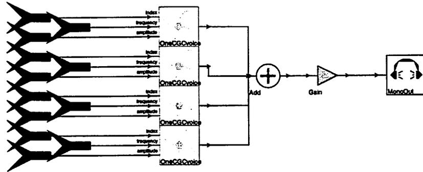
**Figure 5.17** The sound synthesis block of the MIDI synthesizer, described using SDF. Four FM synthesis blocks feed their outputs into an adder that sends its output to a speaker.
