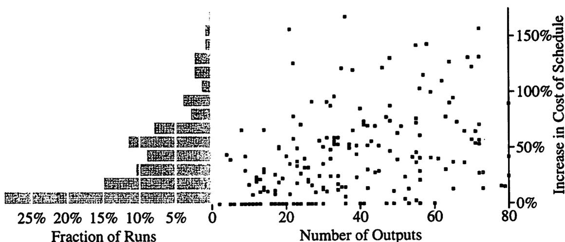
**Figure 4.20** The increase in schedule cost from using the heuristic sweep partition generator.
