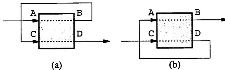
**Figure 2.6** The problem with flattening concurrency. If the order in which the module processes its inputs is fixed, one of these systems will incorrectly deadlock.
