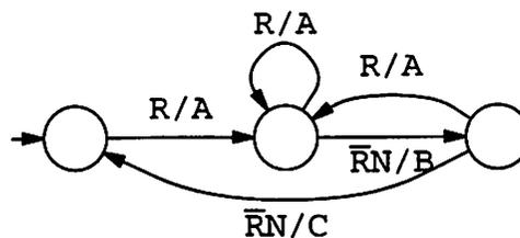
**Figure 2.3** The sequencer example described using a state diagram
