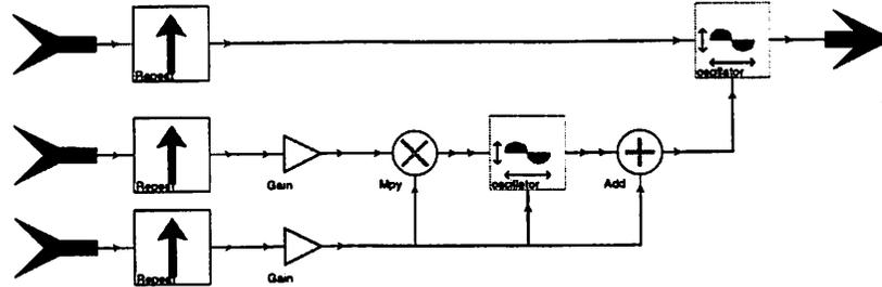
**Figure 5.18** An FM synthesis block. The inputs are an amplitude, a center frequency, and an index of modulation. The modulating frequency is the same as the carrier. The repeat blocks (upward arrows) on each input control the number of samples generated per tick of the enclosing SR domain.
