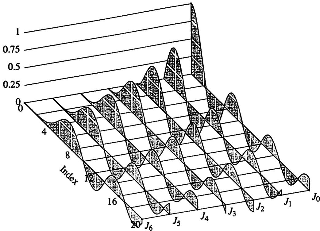
**Figure 5.10** The first seven Bessel functions. For a given index of modulation,  $I$ , the amplitude of the  $k$ th harmonic comes from  $J_k(I)$ .
