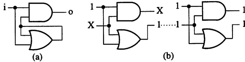
**Figure 3.3** (a) A simple cyclic combinational circuit in which  $o$  follows  $i$ . (b) Malik's procedure for simulating the circuit, showing the output is 1 with when the input is 1.
