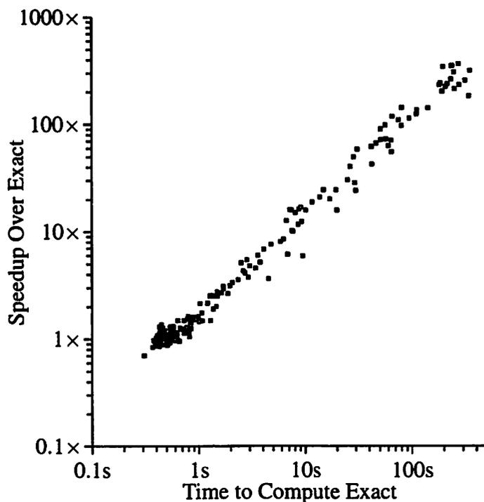
**Figure 4.19** The scheduling time speedup arising from using the heuristic sweep partition generator.
