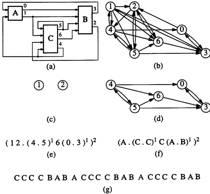
**Figure 4.1** A complete example of scheduling an SR system. (a) The system. (b) Its (strongly connected) dependency graph. (c) The vertices removed by the scheduler to break strong connectivity. (d) The graph that remains. (e) The schedule. Superscripts denote the number of iterations. (f) The schedule after its transformation to block evaluations. (g) The sequence of blocks to evaluate each instant.
