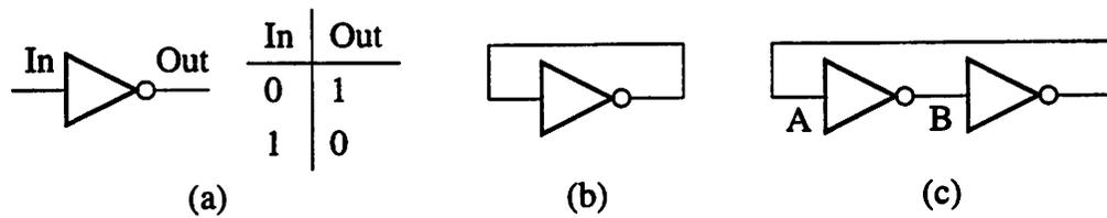
**Figure 3.2** (a) An ideal binary inverter and its truth table. (b) A feedback circuit with no stable states. (c) A feedback circuit with two stable states.
