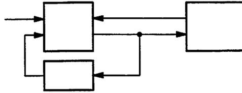
**Figure 1.1** A simple SR system composed of three blocks communicating over three channels. The dangling channel on the left is an input from the environment. Some of the internal channels may be outputs to the environment.
