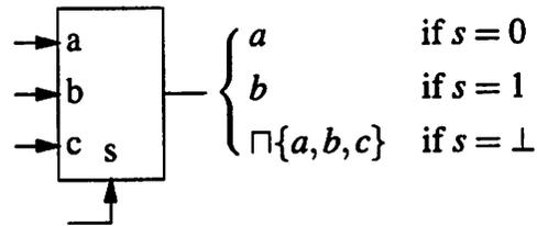
**Figure 6.2** The universal monotonic multiplexer for the binary CPO  $\{\perp, 0, 1\}$ . It is monotonic, so a system constructed solely from these will be monotonic. Moreover, any monotonic function can be built with it.
