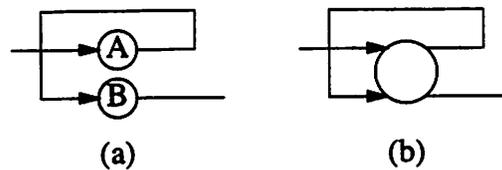
**Figure 6.1** An example of non-compositionality in SDF. (a) A correct system. (b) One that deadlocks after blocks A and B have been encapsulated.
