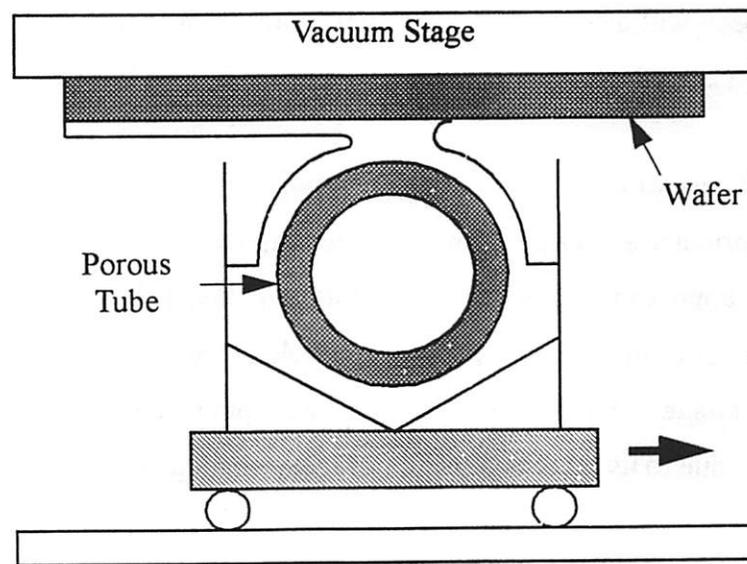
**Figure 2.7** Schematic of the Meniscus Coating Process [14].
