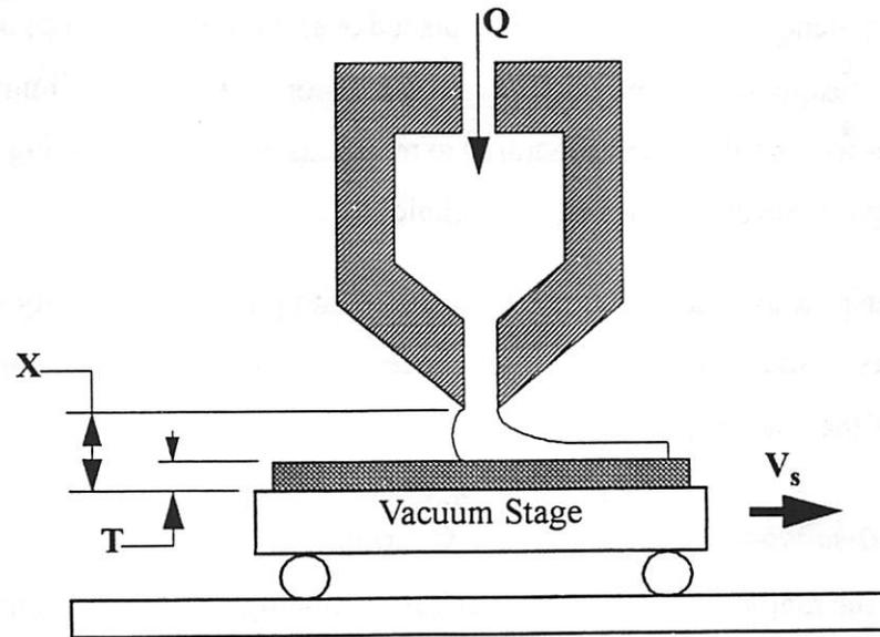
Figure 2.8 Schematic of the Extrusion Coating Process [14].
