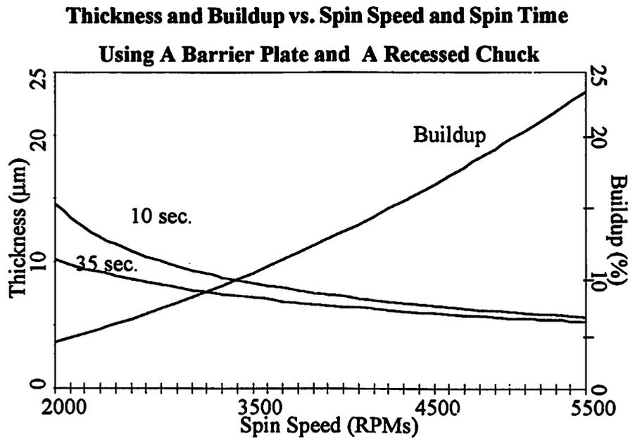
**Figure 4.1** Thickness and Buildup vs. Spin Speed and Spin Time.
