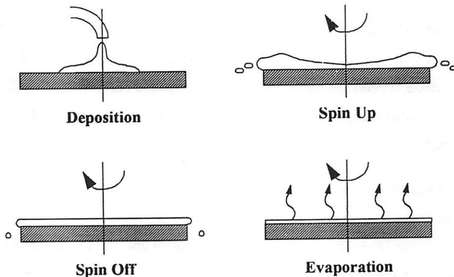
**Figure 2.1** The Four Stages of the Spin Coating Process [7].
