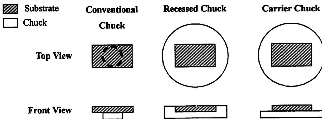
**Figure 3.2** The Three Chuck Types Used For Experiment 1.
