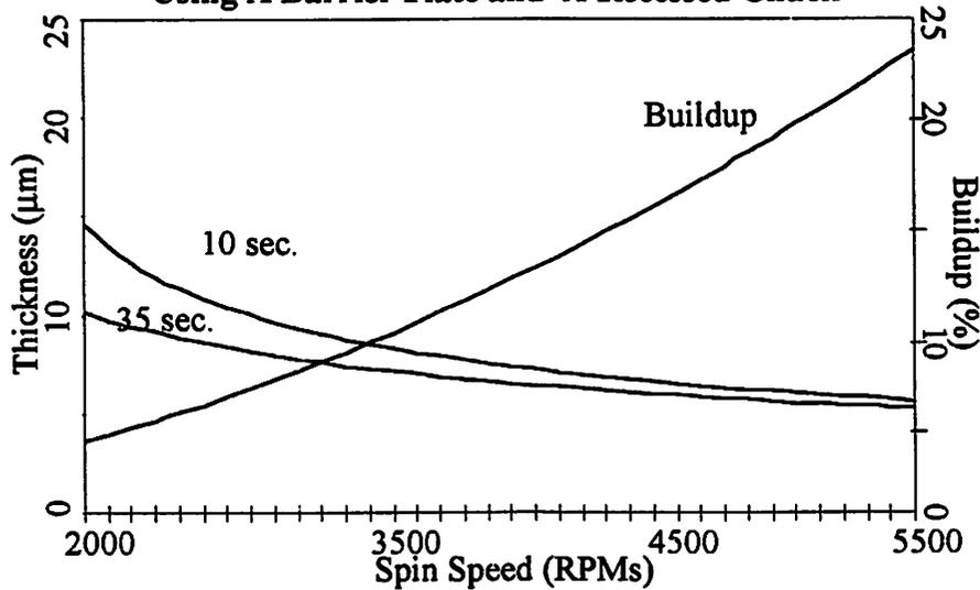
Figure 3.4 Thickness and Buildup vs. Spin Speed and Spin Time.
