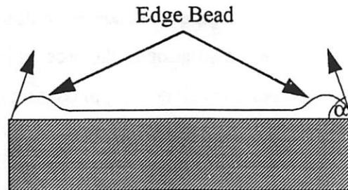
**Figure 2.2** Illustration of the Edge Bead Effect.
