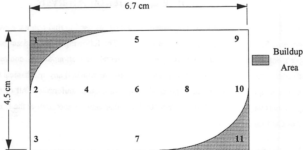
**Figure 3.1** Top View of Rectangular Substrate, Showing the Measurement Locations Used in Experimental Analysis.
