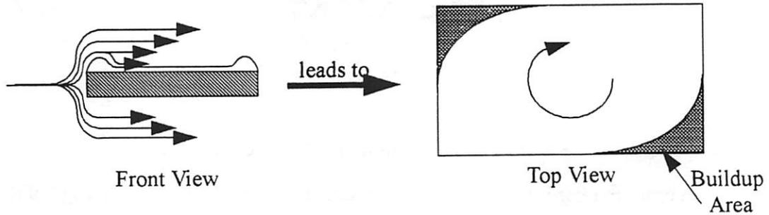
**Figure 2.5** Bernoulli Effect when Spin Coating Rectangular Substrates.
