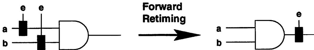
Figure 16: Retiming enabled latch across gates
