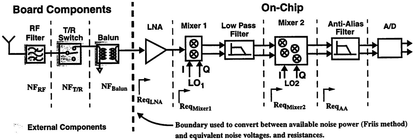
**FIGURE 16. Model showing the boundary for the two step noise calculation.**
