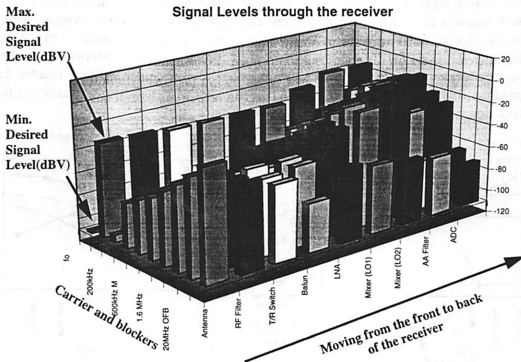
FIGURE 34. All the GSM signal levels in the receiver chain including both inband and out-of-band blockers.
