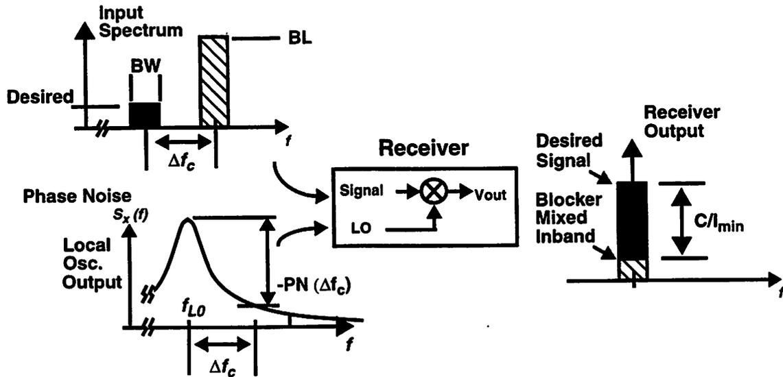
FIGURE 22. Simple calculation for required phase noise performance of the LO.
