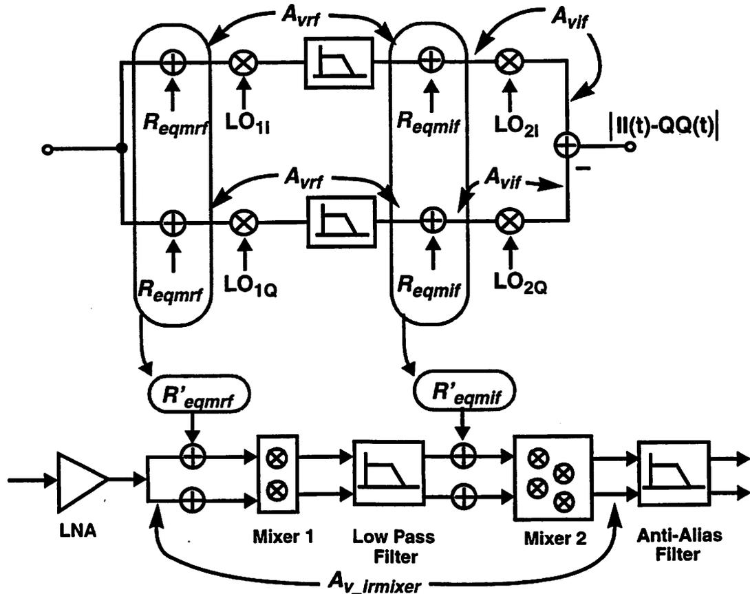
FIGURE 26. Model used to evaluate the noise and single gain in a single channel.
