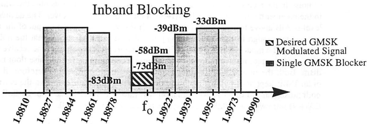
FIGURE 7. DECT Inband blocking requirements
