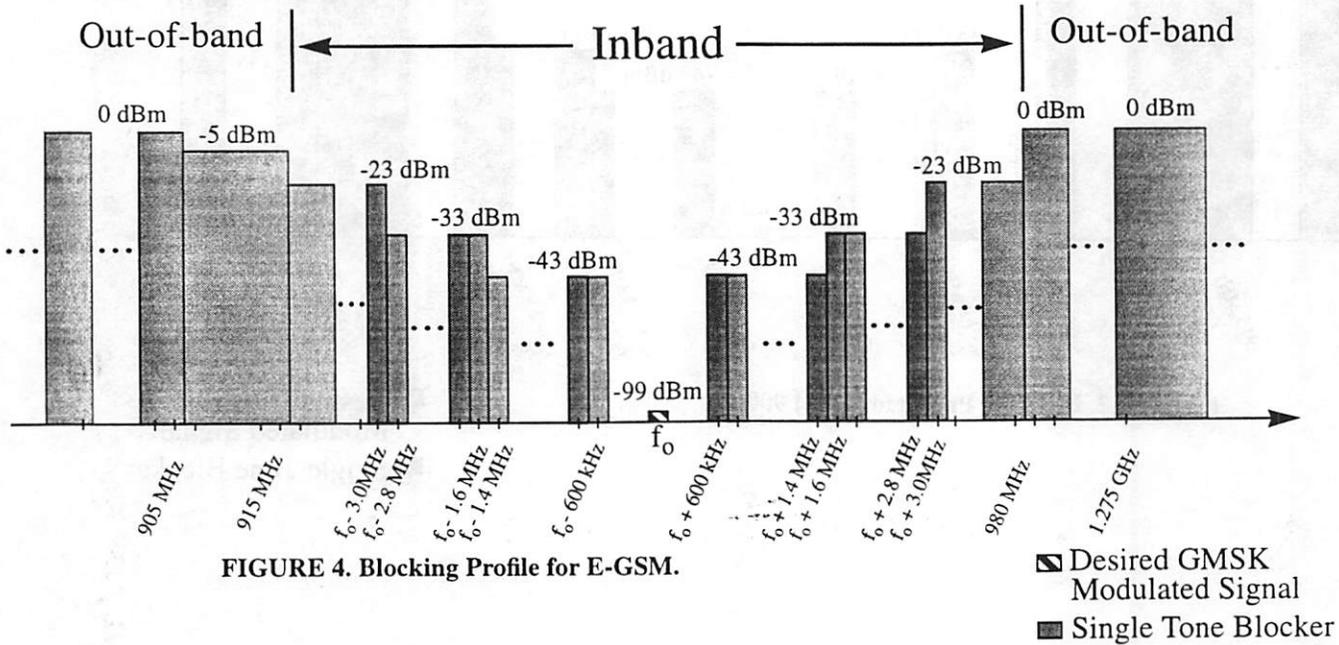
FIGURE 4. Blocking Profile for E-GSM.
