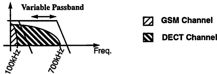
FIGURE 28. Bandwidth channel filtering requirements for dual-standard operation. Both the DECT and GSM channel are frequency translated to baseband.
