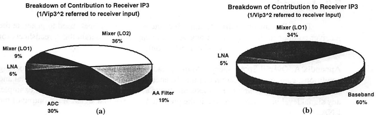
FIGURE 38. Individual contribution of each block to the overall receivers input referred IP3. The breakdown is with respect to each receiver block's  $V_{IP3}$  referred to the receiver input, (a) Wideband IF (b) Low-IF w/ single conversion
