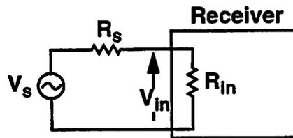
FIGURE 13. Input of the receiver with a source.  $V_{in}$  is the closed circuit voltage while  $V_s$  is the open-circuit voltage.
