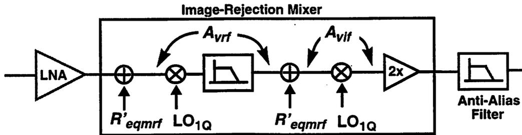
FIGURE 27. Model used to refer the noise of the individual mixers to the overall noise contribution in the receiver.
