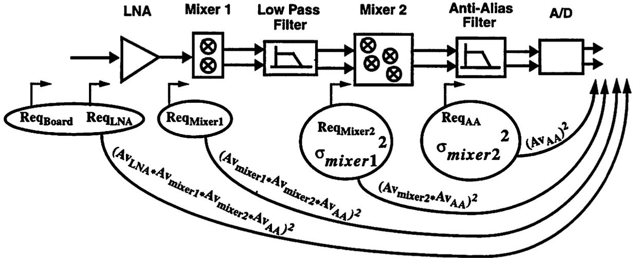
FIGURE 23. Sources of interference in the receiver signal path while an undesired blocker is present.
