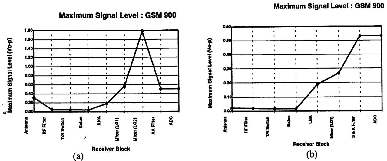
FIGURE 33. Maximum signal levels throughout the receiver chain due to the blockers, (a) Wideband-IF (b) Low-IF with single conversion.
