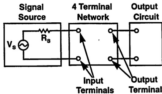
FIGURE 14. Simple Four terminal Network
