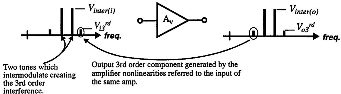
**FIGURE 18. Representation of the adjacent channel interferers and the intermodulated 3rd order component which is created.**
