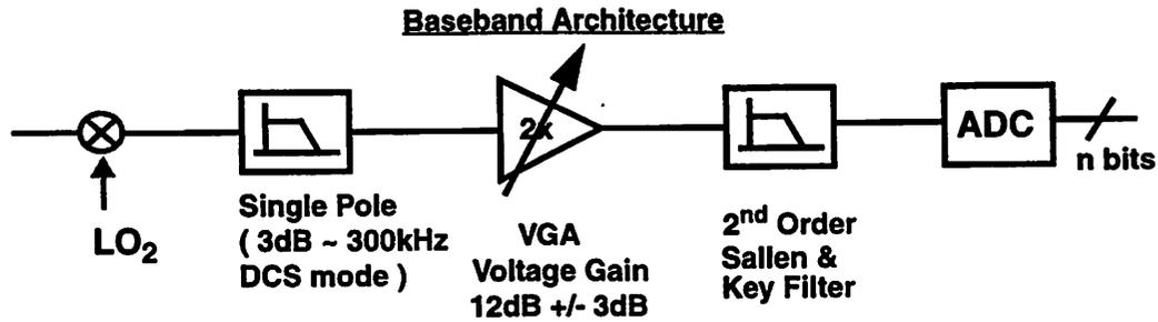
FIGURE 29. Baseband filter and ADC configuration.
