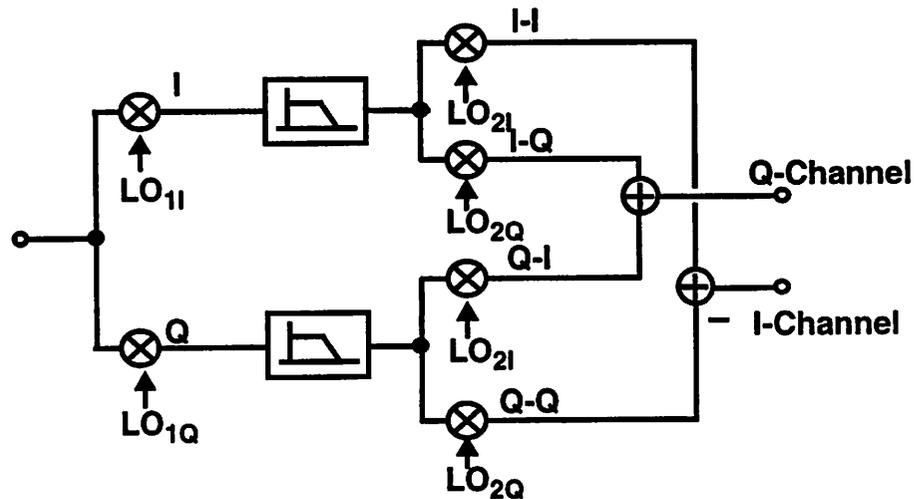
**FIGURE 24.** Weaver Method used to implement the mixing configuration of the wideband IF architecture.
