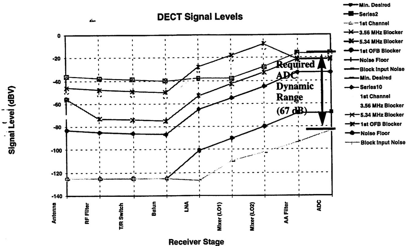
FIGURE 31. All possible DECT signal levels in dBV plotted at the output of each receiver stage.
