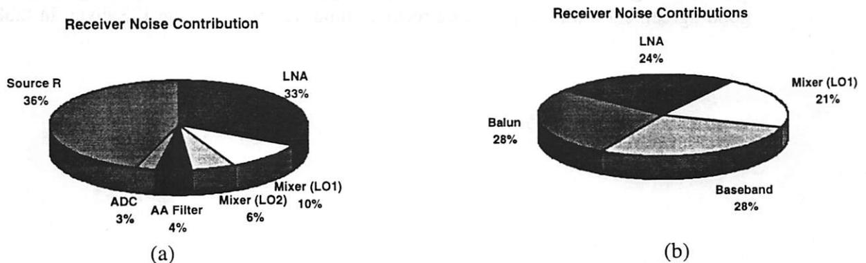
FIGURE 35. Breakdown in the input referred noise contributors from different receiver blocks in (a) Wideband-IF and (b) Low-IF with single conversion.
