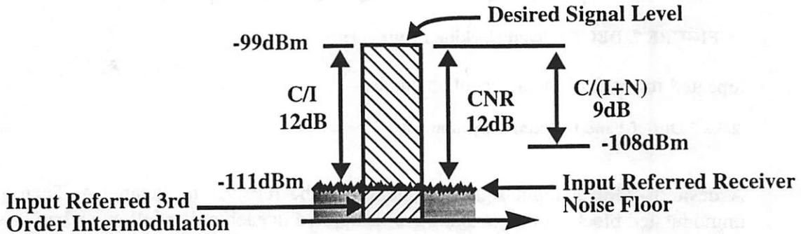
FIGURE 10. Maximum allowable input referred noise and distortion floors under the intermodulation test for GSM, PCS 1900.
