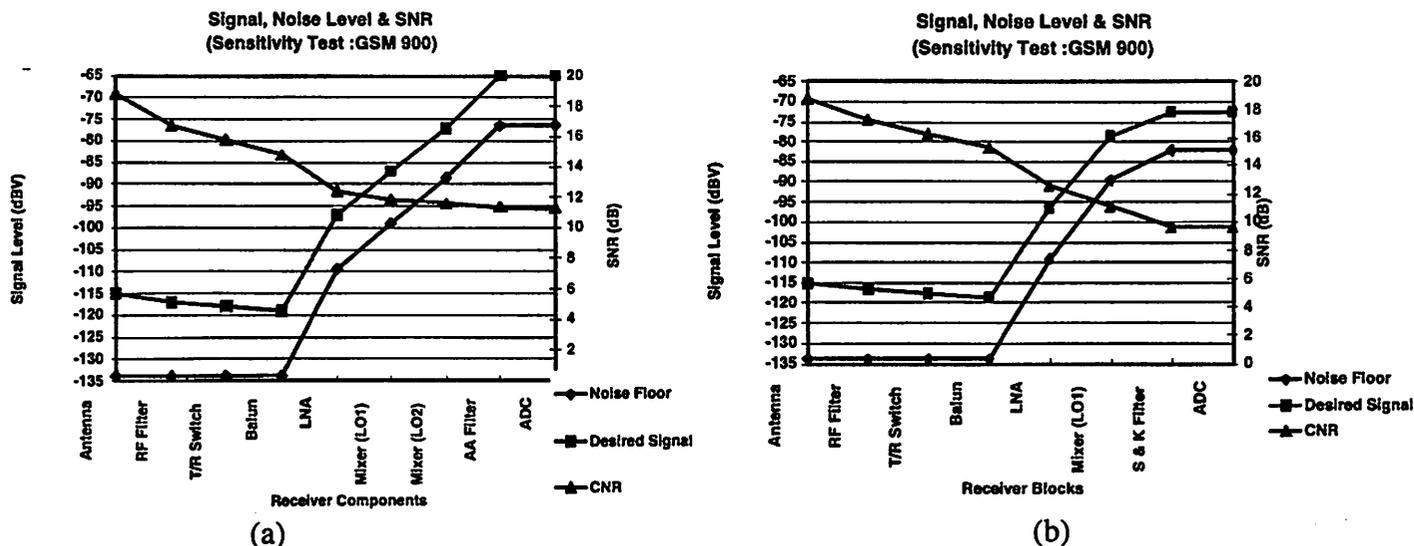
FIGURE 32. Noise floor, minimum signal level and carrier-to-noise ratio CNR in dBV for (a) Wideband IF (b) Low-IF with signal conversion.
