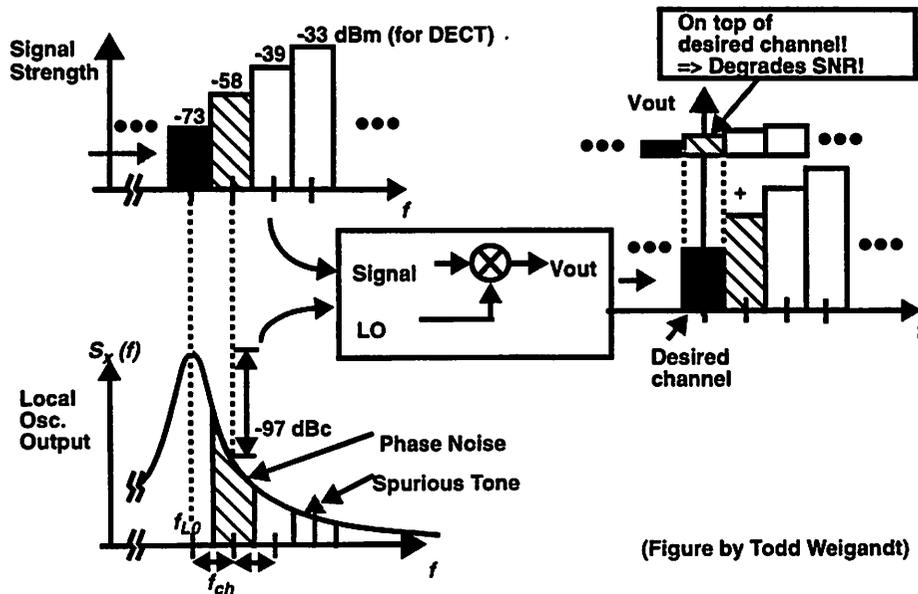
FIGURE 21. Reciprocal mixing of the blocker and phase noise
