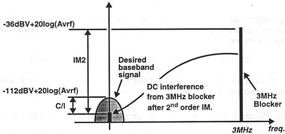
FIGURE 20. Signal spectrum after the second mixer in the wideband IF receiver during the GSM 3MHz blocking test. An interferer is created within the signal band by the 3MHz blocker passing through the baseband 2<sup>nd</sup> order nonlinearities.
