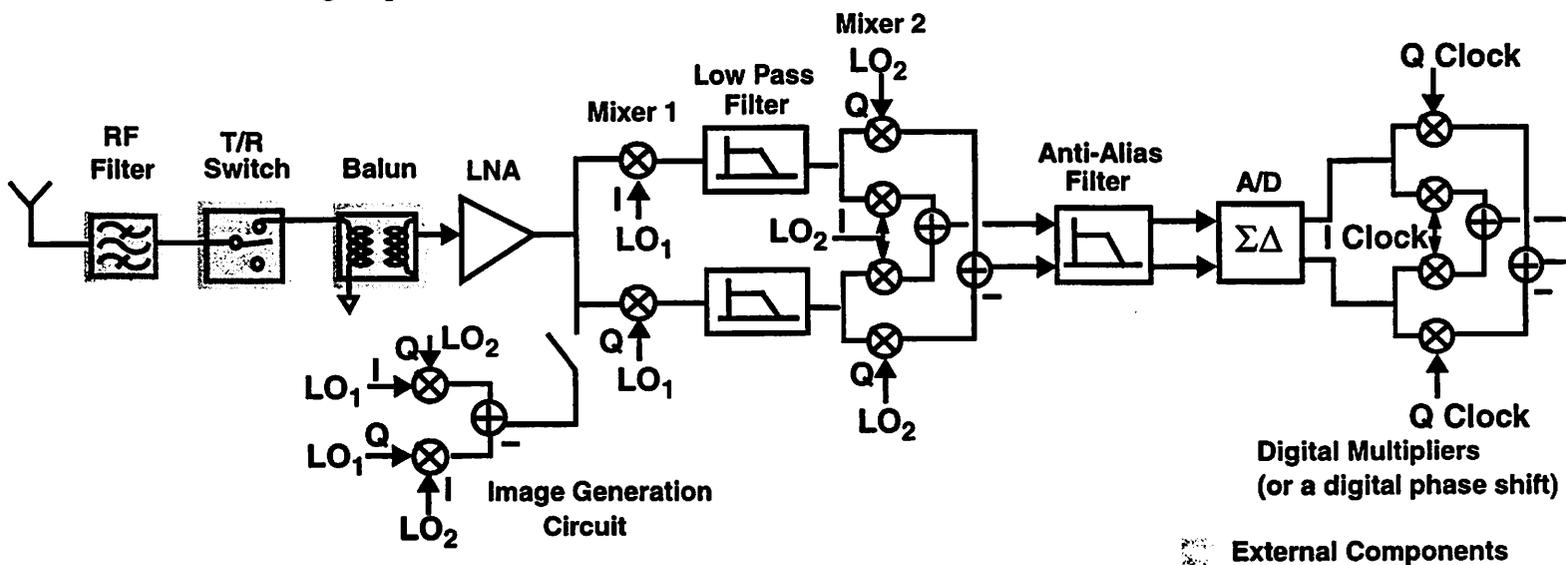
FIGURE 11. Wideband IF w/ Double Conversion Architecture
