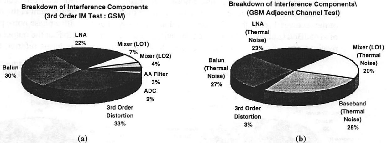
FIGURE 37. Contribution to the overall noise floor at the output of the receiver including the 3<sup>rd</sup> order distortion components created by two (-49 dBm) intermodulating tones (a) Wideband IF (b) Low-IF with single conversion.
