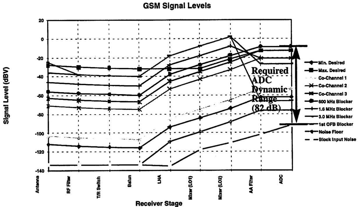
FIGURE 30. All possible GSM signal levels plotted at the output voltage of each receiver stage.
