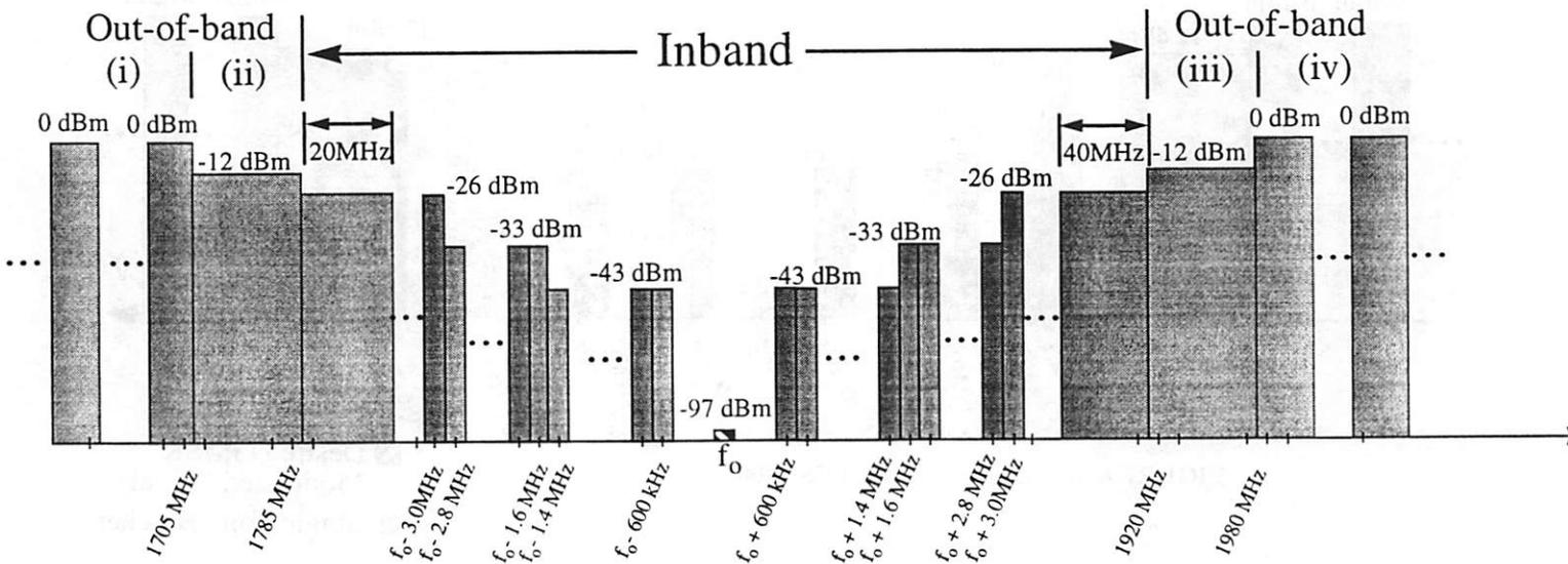
FIGURE 5. Blocking profile for DCS 1800.
