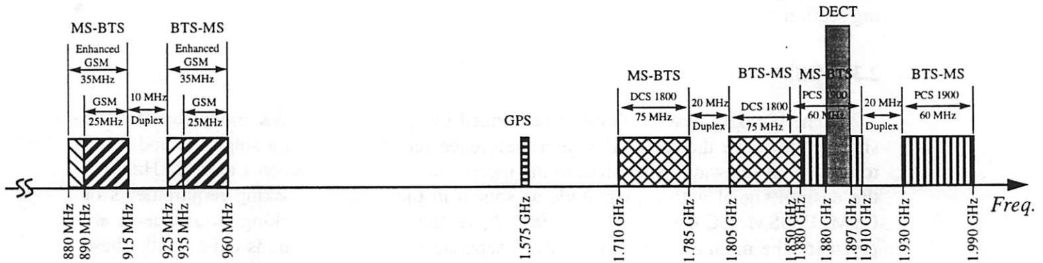
FIGURE 1. Frequency Bands of interest for the (GSM / DECT / GPS) Receiver.
