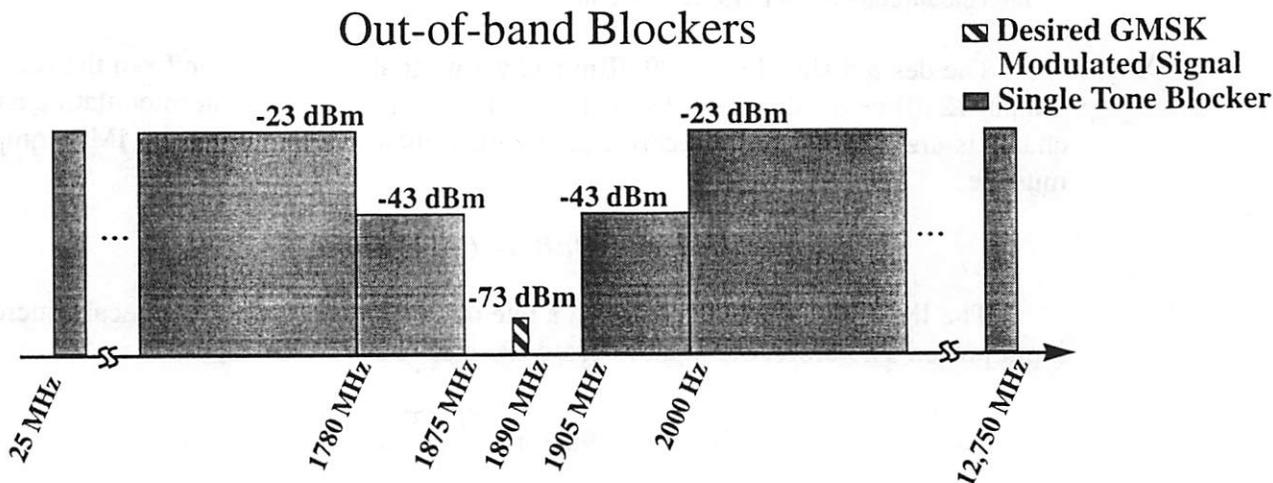
FIGURE 9. Out-of-Band DECT blocking requirements.
