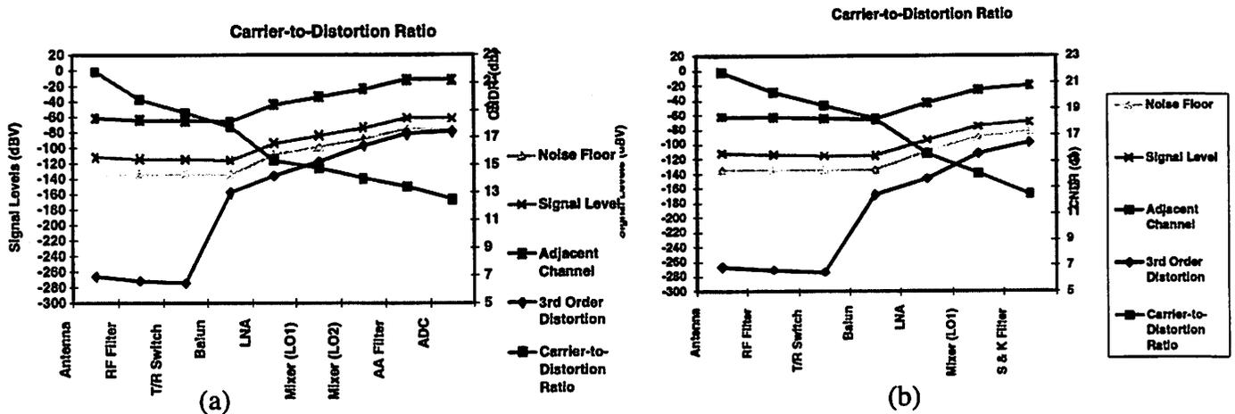
FIGURE 36. The desired signal level, noise floor, 3rd Order distortion components, adjacent channel signal strength all dBV are plotted with respect to the left axis for each stage down the receiver chain. The right axis shows the carrier-to-(noise + distortion) ratio for both (a) Wideband IF and (b) Low-IF with single conversion.
