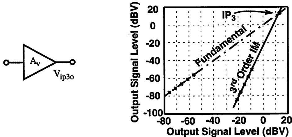
FIGURE 17. Simple Amplifier with voltage gain  $A_v$  and Output Third order intercept  $V_{ip3o}$
