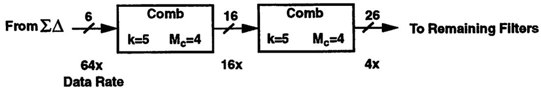
Fig. 3.11: Comb Filter With Two-Stage Implementation
