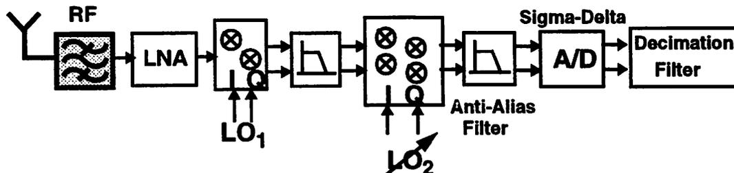
Fig. 2.4: Wide-Band IF Double Conversion Receiver
