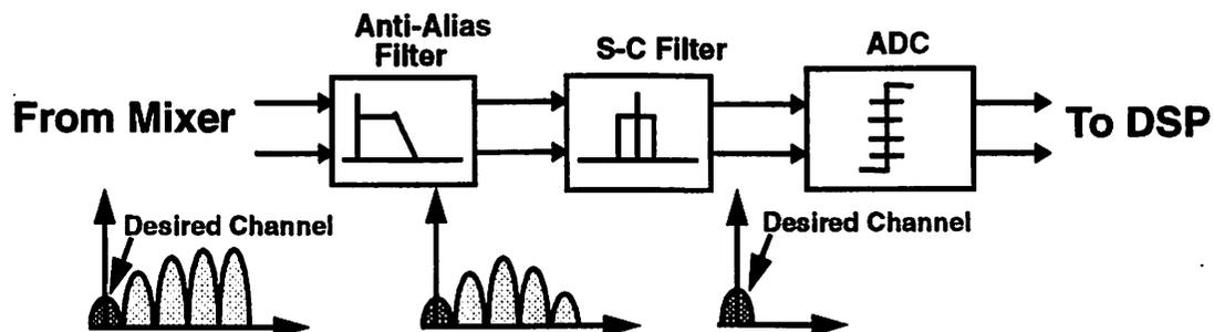
Fig. 2.6: Analog Channel Select Filtering
