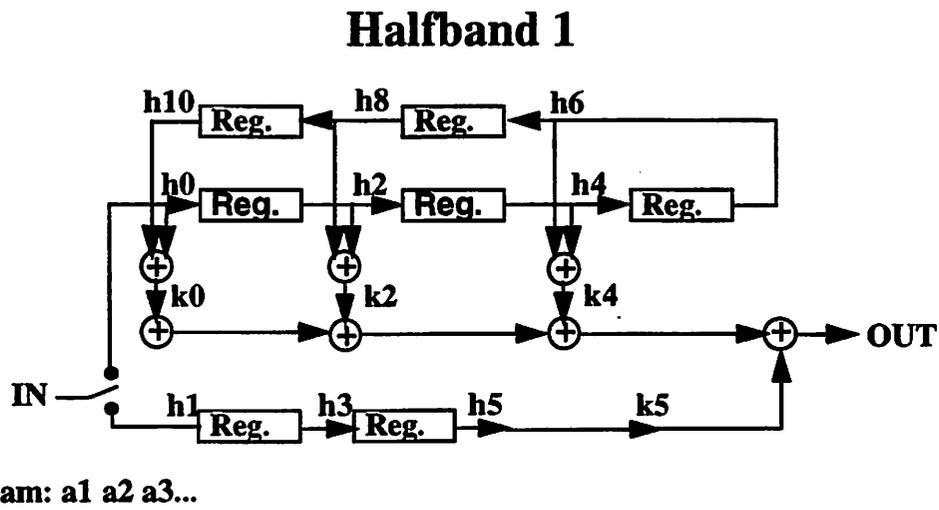
Fig. 4.10: Direct-Form Polyphase Implementation of Halfband 1
