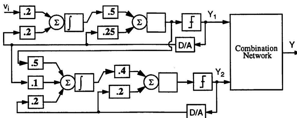
Fig. 2.12: Sigma-Delta Architecture
