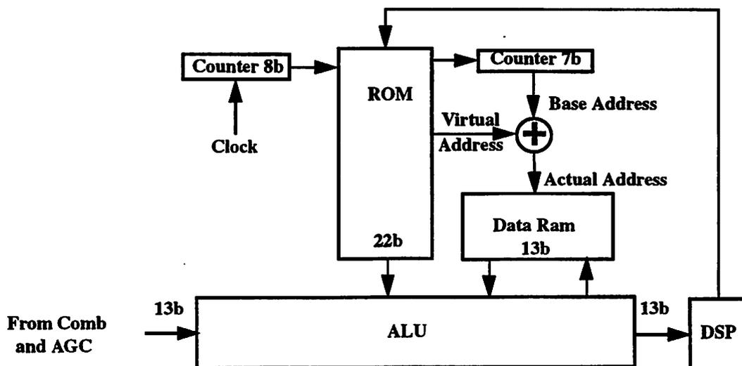
Fig. 4.5: Architecture of ROM Mask-Programmable Implementation [24]
