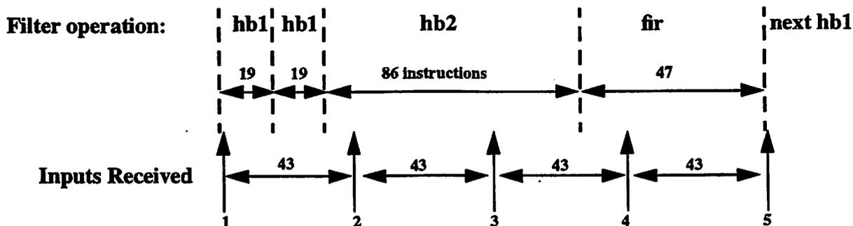
Fig. 4.7: Incorrect ROM Ordering of Filter Operations
