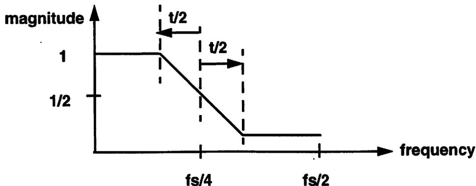
Fig. 3.6: Magnitude Response of a Halfband Filter
