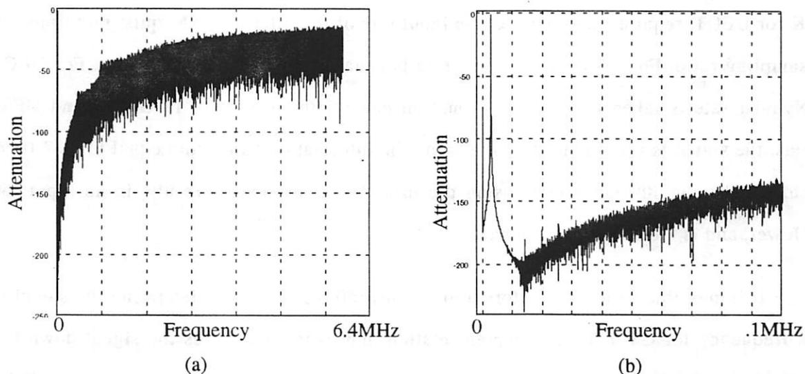
Fig. 2.13: Worst Case Quantization Noise at the Sigma-Delta Output (a) entire spectrum
