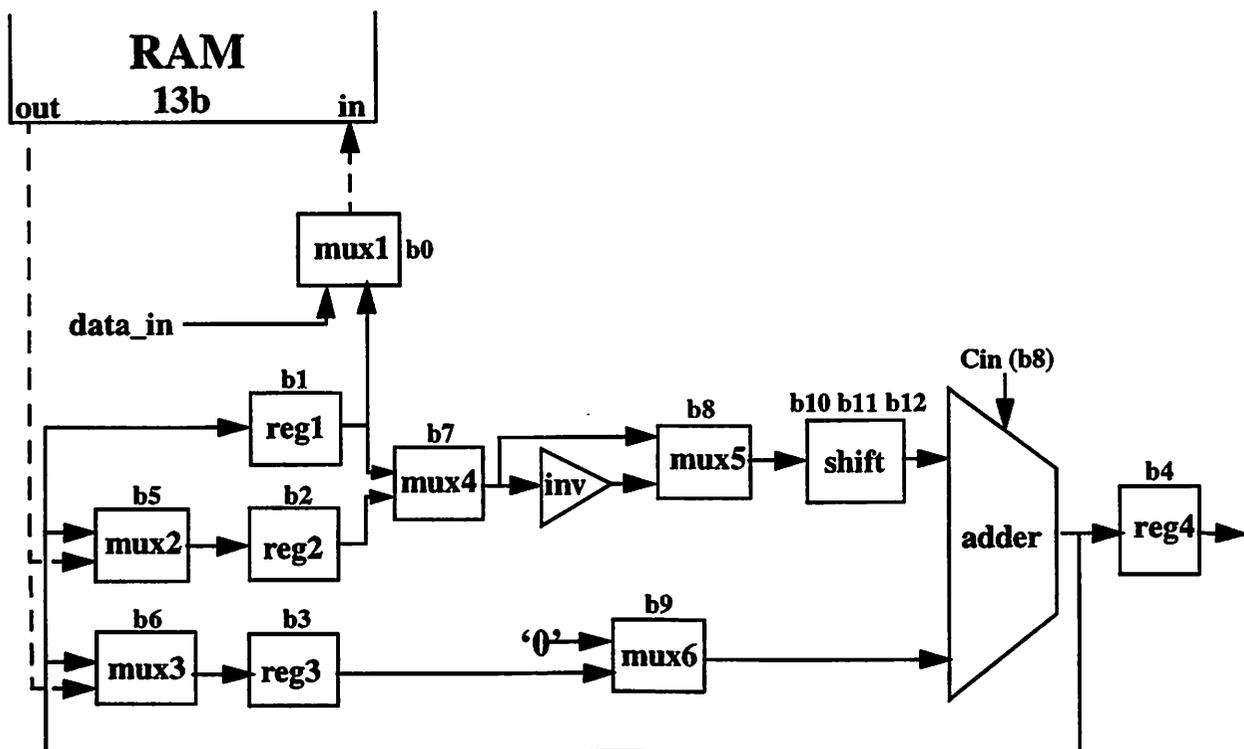
Fig. 4.6: Block Diagram of Arithmetic Unit [24]
