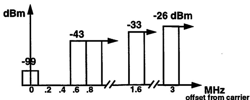
Fig. 2.8: GSM Blockers
