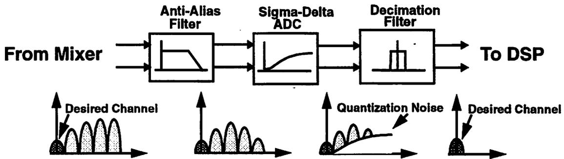
Fig. 2.7: Digital Channel Select Filtering
