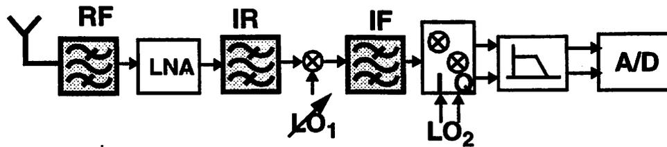
Fig. 2.1: Super-Heterodyne Receiver
