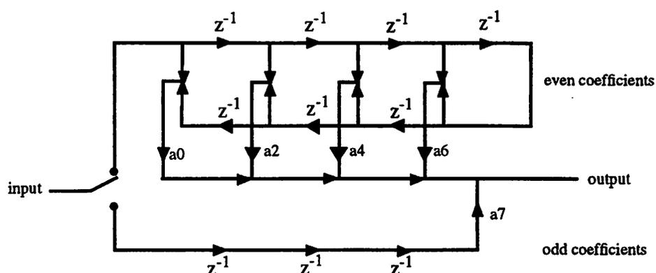
Fig. 3.7: Polyphase Direct-Form Implementation of a 14-tap Halfband Filter
