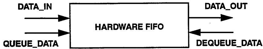
Figure 2.19 An interface model of a hardware FIFO.
