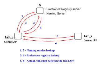
Figure 14: The Setup for Latency Measurements
