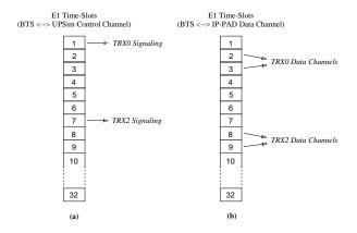
Figure 11: E1 Time-Slots used for signaling and data
