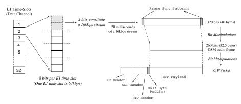
Figure 12: The Conversion of GSM frames to RTP Packets at the IP-PAD
