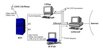
Figure 10: An IAP interfaced to the GSM network
