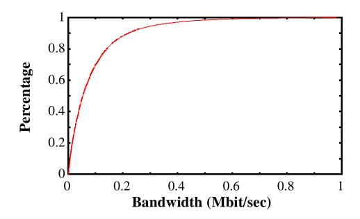
Figure 5.2: CDF of measured bandwidth for for transfers between clients at IBM Research and servers in the Internet
