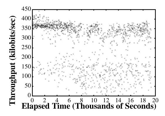
Figure 3.7: Scatter plot of throughput from IBM to UC Berkeley over a 5 hour period.
