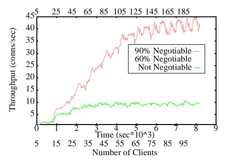
Figure 5.15: Apache throughput for varying fractions of negotiable bytes
