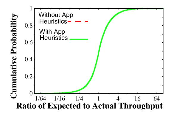
Figure 4.8: CDF of ratio of expected throughput (as generated by the performance server) to actual throughput (as reported by the client). The X axis is on a log scale.
