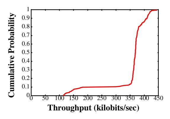
Figure 3.8: CDF of throughput from IBM to UC Berkeley: initial 30 minutes.
