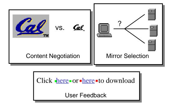
Figure 1.1: Examples of Application Level Adaptation.
