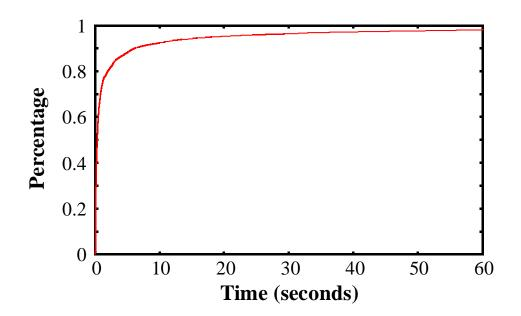
Figure 5.1: CDF of measured transmission times for pages retrieved by clients at IBM Research from servers in the Internet
