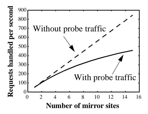
Figure 3.3: The effect of probe traffic on scalability. Figure shows requests/second that mirrors can serve as a function of the number of mirror sites.
