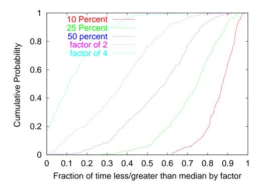
Figure 3.10: Quantifying network noise. Figure shows likelihood of being more F away from median performance for a given client-server pair.
