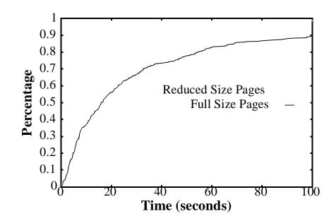
Figure 5.8: CDF of transmission times for pages that had performance estimates and required an alternate version. Retrieval times for the original page and the alternate version are shown.
