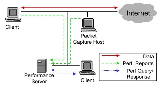
Figure 4.1: Components of SPAND.
