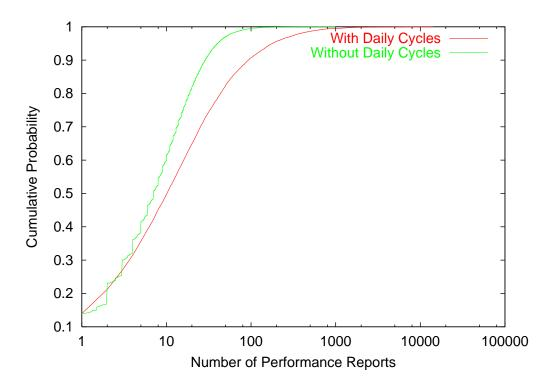
Figure 4.9: Distribution of number of performance reports for a given distant host when daily cycles are and are not taken into account. The X axis is on a log scale.
