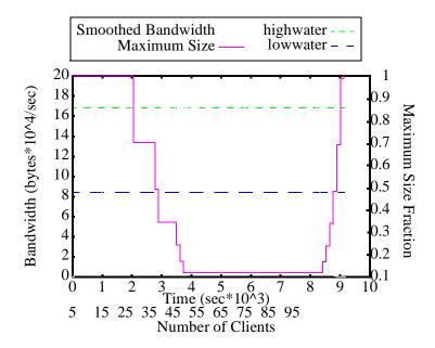
Figure 5.12: Bandwidth leaving Apache as a function of number of clients with content negotiation
