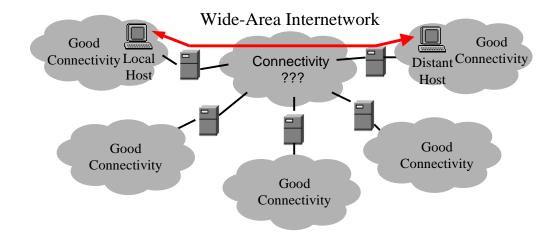
Figure 3.1: Network Model behind SPAND. Local Hosts in well connected domain communicate with distant hosts through an Internetwork, the properties of which are unknown.
