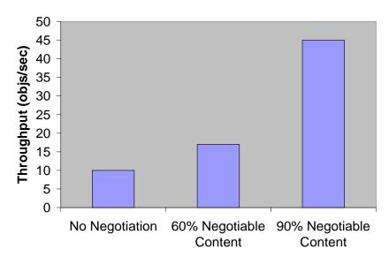
Figure 1.4: Maximum web server throughput with Surge workload and varying amounts of Content Negotiation.
