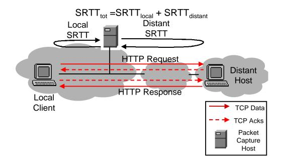
Figure 4.4: How SRTT is measured at the packet capture host.
