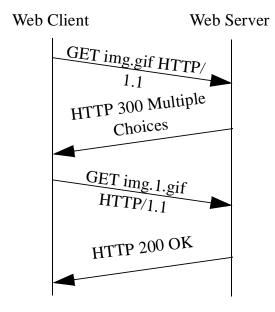
Figure 5.4: Sample transaction using transparent content negotiation
