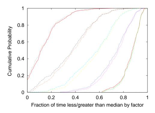
Figure 3.11: Quantifying sharing noise. Figure shows likelihood of being more than F away from median performance for a given (group of clients, server) pair.
