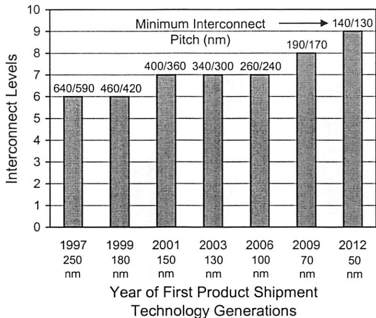
Figure 1.4 Present and projected interconnect levels and minimum contacted/non-contacted interconnect metal pitch of logic circuits for different technology nodes and year of first product shipment as per NTRS [13].
