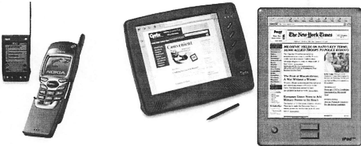
Figure 1.1. Wireless devices, from low-bandwidth to high-bandwidth: The Palm VII, Nokia 7110 cell phone, National Semiconductor WebPAD, artist's rendering of an InfoPad prototype.
