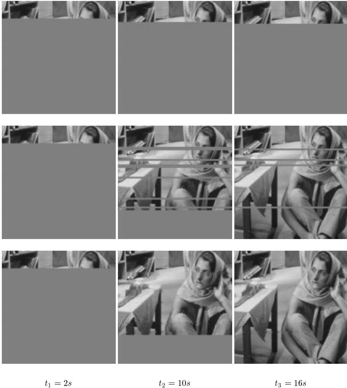
Figure 6.8: Snapshots of the displayed image with a TCP-like transport (first row), with ITP (second row), and with ITP enhanced with error concealment (last row) at 10% loss rate. The entire transfer of the 184 KB image takes 16.57s to complete.
