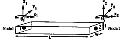
Figure 1: The atomic element description of a beam. The geometric variables, L, w, t , correspond to design variables. The displacements x_1, y_1, \theta_1, x_2, y_2, \theta_2 are related to the design specification and performance parameters.
