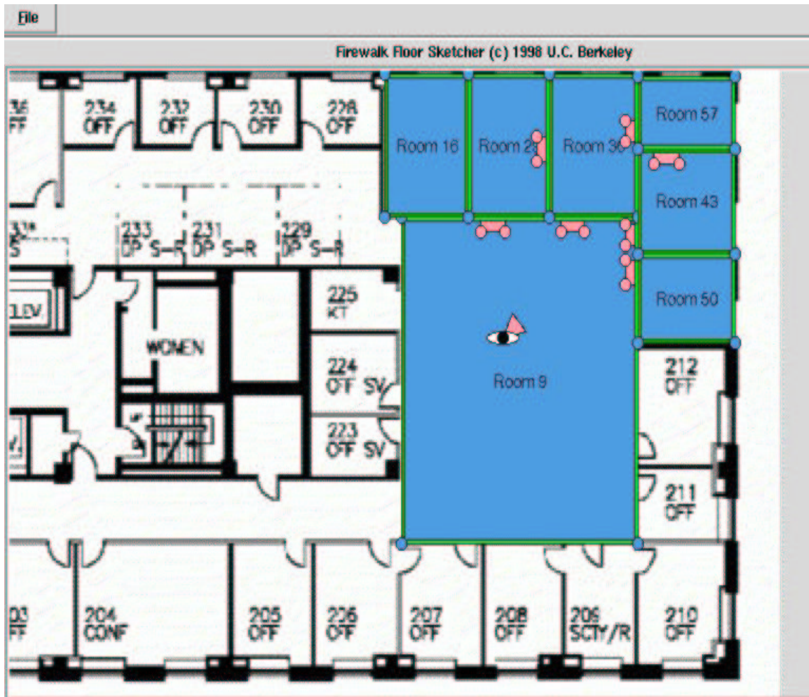
Figure 6.6: Using a JPEG image in the background, the user can more easily “trace” an existing floorplan into a 3D model.
