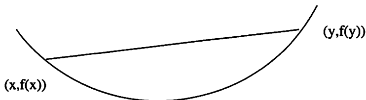
Figure 3.1: Graph of a convex function, where the chord between two points lies above the graph
