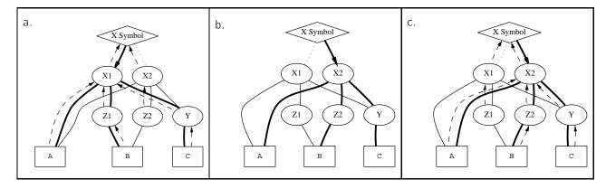
Figure 12: Changes in alternatives require changes in parent links. In (a), X1 is the primary alternative. If X2 rather than X1 is chosen as the primary alternative for the symbol node (bold arrow in b), the membership of the primary subtree changes (bold edges in b), and corresponding changes are needed in the primary parent pointers (dashed arrows in c).
