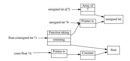
Figure 14: C's types are represented by linked data structures eventually pointing back to a set of basic types.
