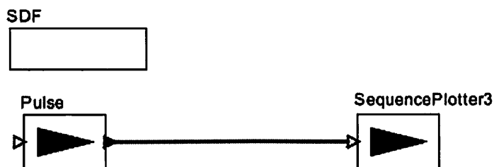
FIGURE 17.6. A model that plots the values of a signal. 256 iterations must be executed to plot the entire signal.
