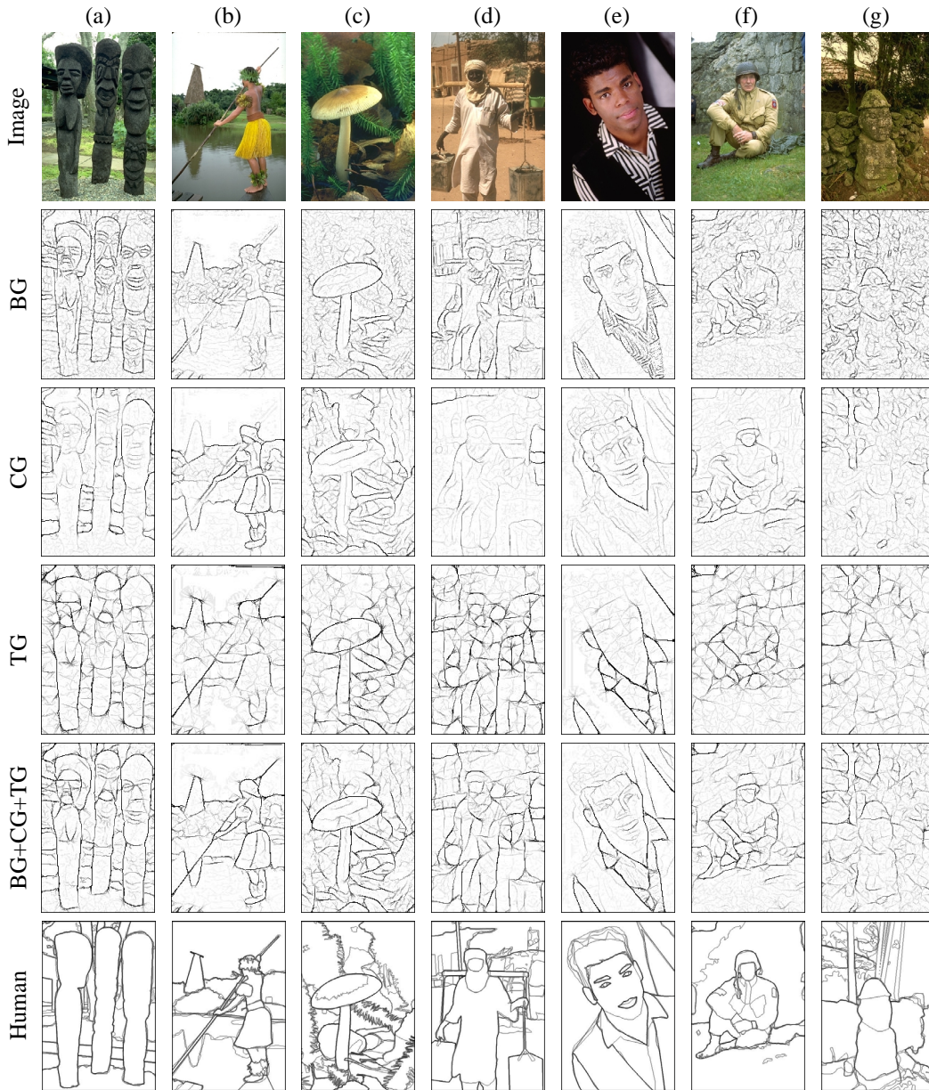
Figure 4.18: Boundary Images for Our Detectors. Rows 2 to 4 show real-valued probability-of-boundary ( P_b ) images after non-maxima suppression for the three cues. The complementary information in each of the three BG, CG, and TG channels is successfully integrated by the logistic in row five. The boundaries in the human segmentations shown in the last row are darker where more subjects marked a boundary.
