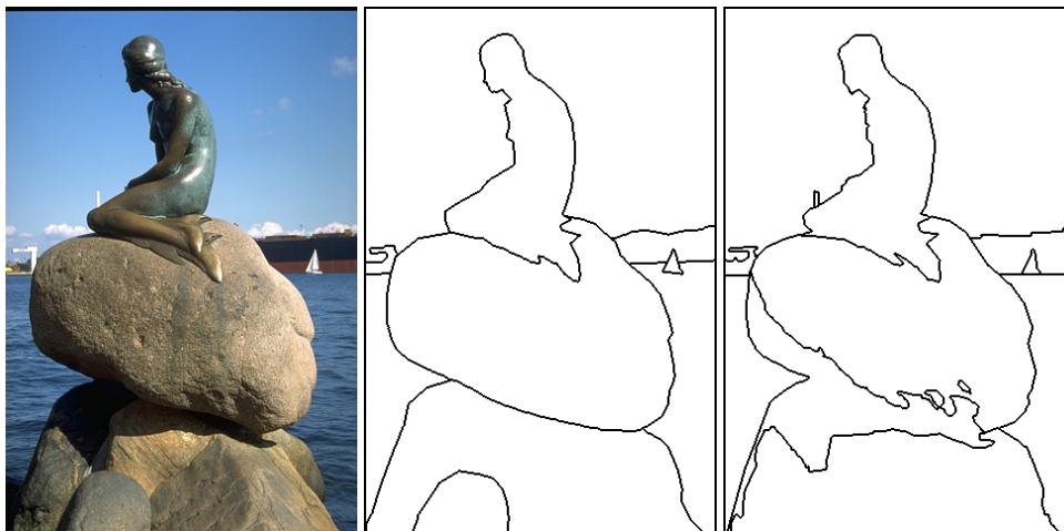
Figure 2.12: Example of Inconsistent Segmentations. This figure shows two additional segmentations of the image used in Figure 2.11. In this case, the two segmentations are not consistent with one another because there is no single hierarchical decomposition of the scene that can explain both. The inconsistency is manifested as overlapping, rather than nested, segments. The right subject's shadow segment spans two rock segments in the left subject's segmentation.
