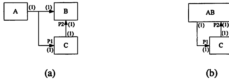
Figure 2.3 Deadlock introduced by composing actor A and B into one composite actor.
