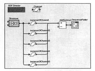
FIGURE 2.37. The model from figure 2.36 with the icon changed for the class. Note that changes to the base class propagate to the instances.
