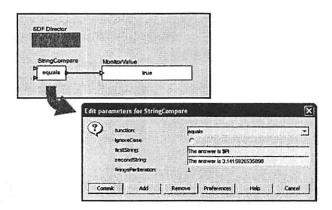
FIGURE 3.4. String parameters are indicated in the parameter editor boxes by a light blue background. A string parameter can include references to variables in scope with *\$name*, where *name* is the name of the variable. In this example, the built-in constant \$PI is referenced by name in the first
