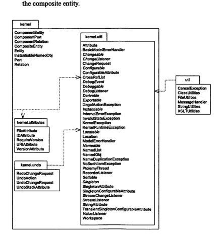
FIGURE 1.12. The kernel package and related packages shown here support the data model (the "abstract syntax") of Ptolemy II designs, which includes the structure of components, their interconnections, and their interrelationships as classes, subclasses, and instances.
