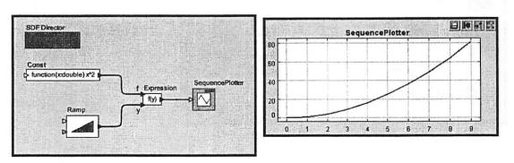
FIGURE 3.6. Example of a function being passed from one actor to another.
