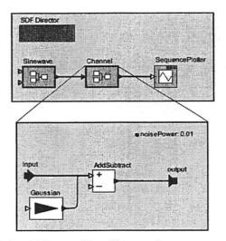
FIGURE 2.34. Hierarchical model that we will modify to use classes.
