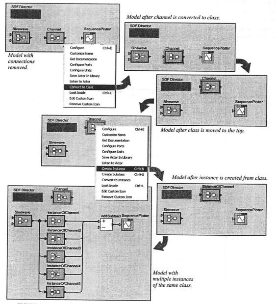
FIGURE 2.36. Creating and using a channel class.
