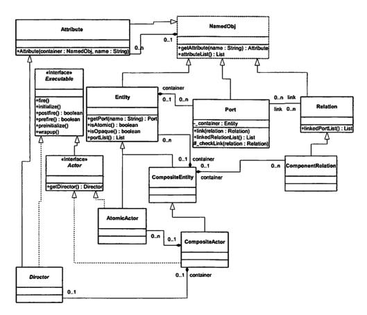
FIGURE 1.21. Simplified static structure diagram for some Ptolemy II classes. This diagram illustrates features of UML syntax that we use. grams, the only constructors available for a class are those shown in the box defining the class. Figure 1.21 does not show all the constructors of these classes, for simplicity.
