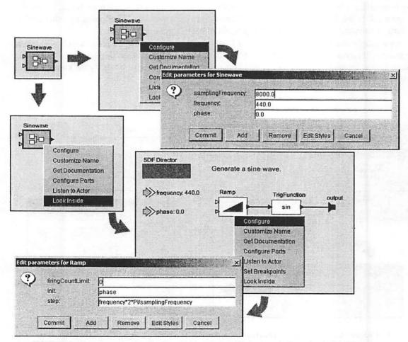
FIGURE 3.3. Sinewave actor, showing its port parameters, and their use at the lower level of the hierarchy.
