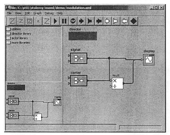
FIGURE 7.12. Rendition of the modulation model in Vergil.
