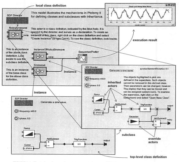
FIGURE 1.4. Illustration of actor-oriented classes, subclasses, and inheritance.
