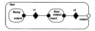
FIGURE 7.7. Sine wave generator topology.
