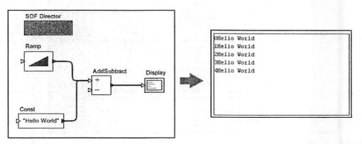
FIGURE 2.19. Addition of a string to an integer.
