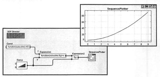
FIGURE 3.7. More elaborate example with functions passed between actors.
