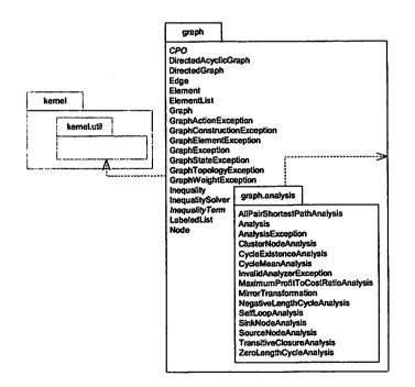
FIGURE 1.15. The graph package and related packages shown here provide graph-theoretic algorithms that operate on the Ptolemy II data model (figure 1.12) to support of static analysis and scheduling.
