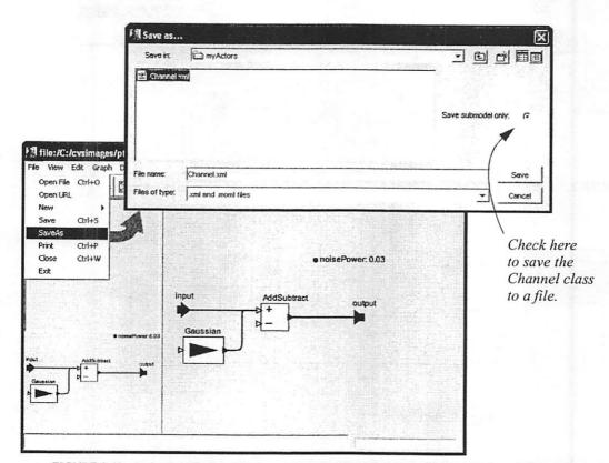
FIGURE 2.42. A class can be saved in a separate file to then be shared among multiple models.
