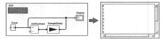
FIGURE 2.50. An SDF model with a feedback loop must have at least one instance of the SampleDelay actor in it.
