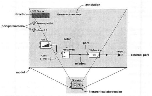
FIGURE 1.2. Illustration of an actor-oriented model (above) and its hierarchical abstraction (below).
