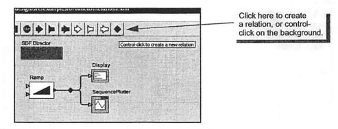
FIGURE 2.15. A relation can be used to broadcast an output from a single port.
