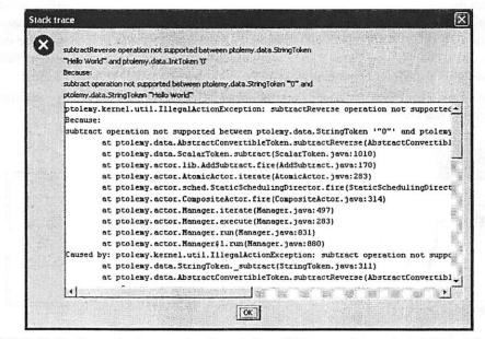
FIGURE 2.18. Stack trace for the exception shown in figure 2.17.
