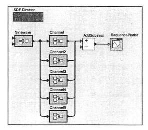
FIGURE 2.35. A poor design of a diversity communication system, which has multiple copies of the channel as defined in figure 2.34. we have modified the custom icons so that each has a different color, and the fifth one has an extra graphical element. To do this, just right click on the icon of the instance and select "Edit Custom Icon."
