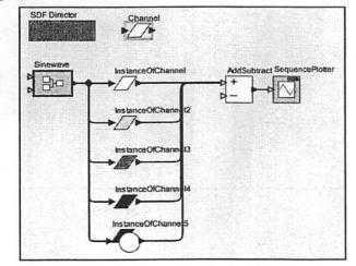
FIGURE 2.38. The model from figure 2.37 with the icons of the instance changed to override parameter values in the class.
