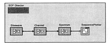
FIGURE 2.48. A multirate SDF model. The *Spectrum* actor requires 256 tokens to fire, so one iteration of this model results in 256 firings of *Sinewave, Channel*, and *SequencePlotter*, and one firing of *Spectrum*.
