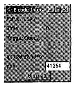
The window presents basic information about the state of the E machine. To run the simulation press the "Simulate" button and the E Machine will start executing the E code. You can stop the execution at any time by pressing the button again (now labeled "Stop").
