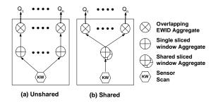
Fig. 4. Possible plans for multiple queries
