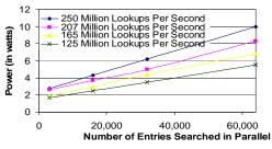
Figure 2. Power consumption for a 9Mbits TCAM.
