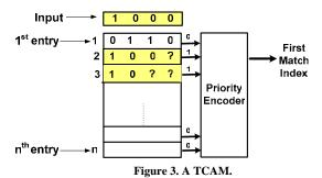
However, TCAMs have some limitations. TCAMs cost about 30 times more per bit of storage than DDR SRAMs [9]. In addition, TCAMs consume 150 times more power per bit than SRAMs. TCAM power consumption grows linearly with the number of entries searched in parallel and is also directly related to the number of TCAM accesses, as mentioned in Section 1.
