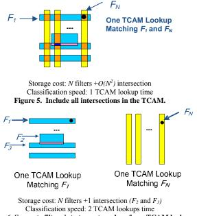
Figure 6. Separate filters into two sets and perform TCAM lookups separately.
